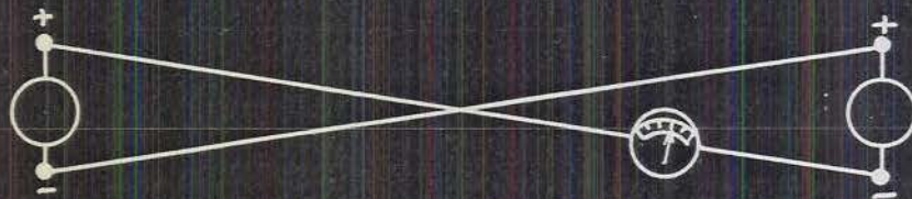
CIRCUIT #3 - PHOTOCELLS IN PARALLEL - METER IN PARALLEL.
