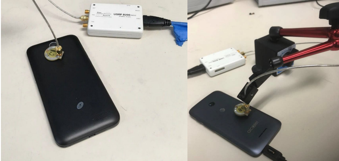
Figure 2: Experimental setup for capturing EM emanations from ZTE ZFIVE (left) and Alcatel Ideal (right) phones. In each setup, our custom probe (the flat, beige, circular object at the end of the silver-colored cable) is positioned close to but not touching the phone. The cable is held in position by a mechanical arm, which is visible in the photo on the right. An Ettus B200-mini SDR (white box) digitizes the signal and sends it through a USB cable to a personal computer (not shown) for analysis.
