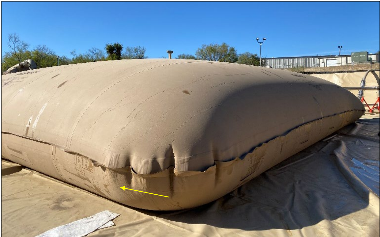
Figure A-6. BLSS #1 (NAFT #1) CFT with Widespread Fuel Leaks and Spotting
