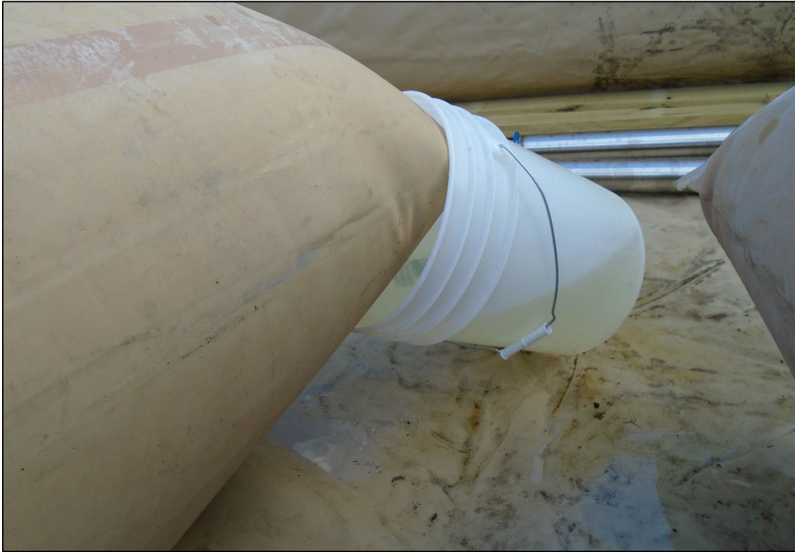
Figure E-5. AEF #5 CFT Fuel Drip from Corner Collected in Bucket
