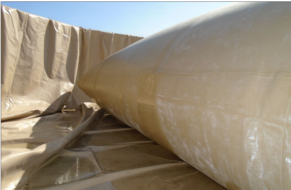
Figure D-6. MILPAWS #4 CFT Fuel Seeping from Seam
