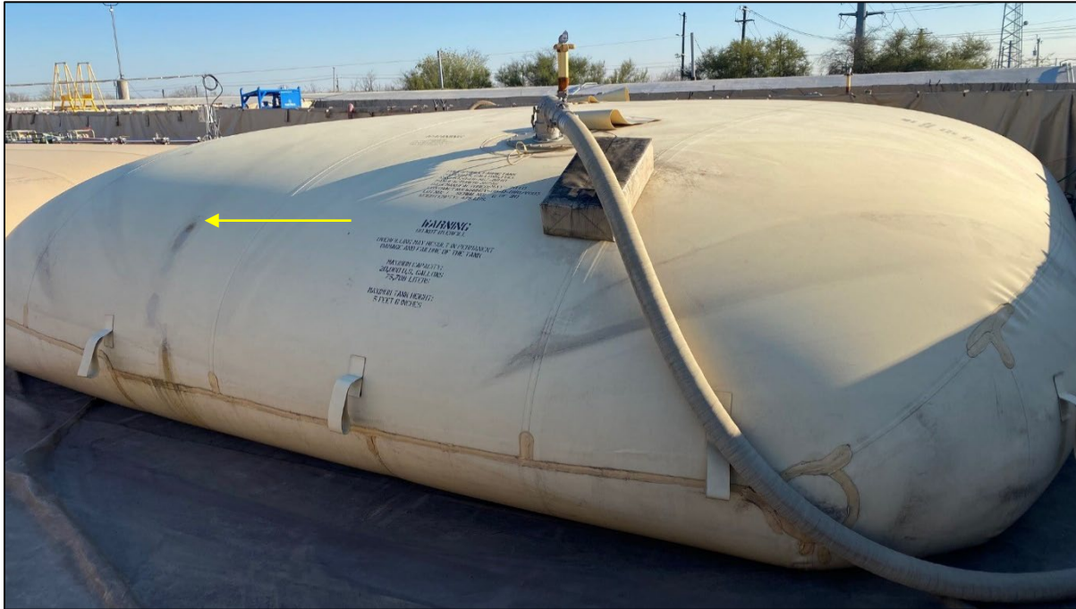
Figure F-4. MPC #6 CFT Showing Surface Fuel Staining
