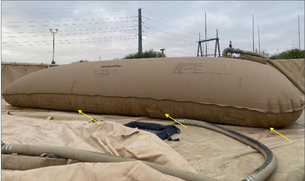
Figure A-8. BLSS #1 (NAFT #1) CFT Spread of Fuel Drips Along Entire Seam
