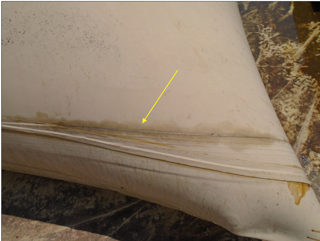
Figure G-4. GTA Spiral #7 CFT Fuel Leaks Along Spiral Seams
