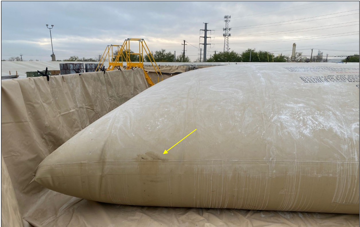
Figure C-5. AEF #3 CFT Developing Fuel Leak at Seam
