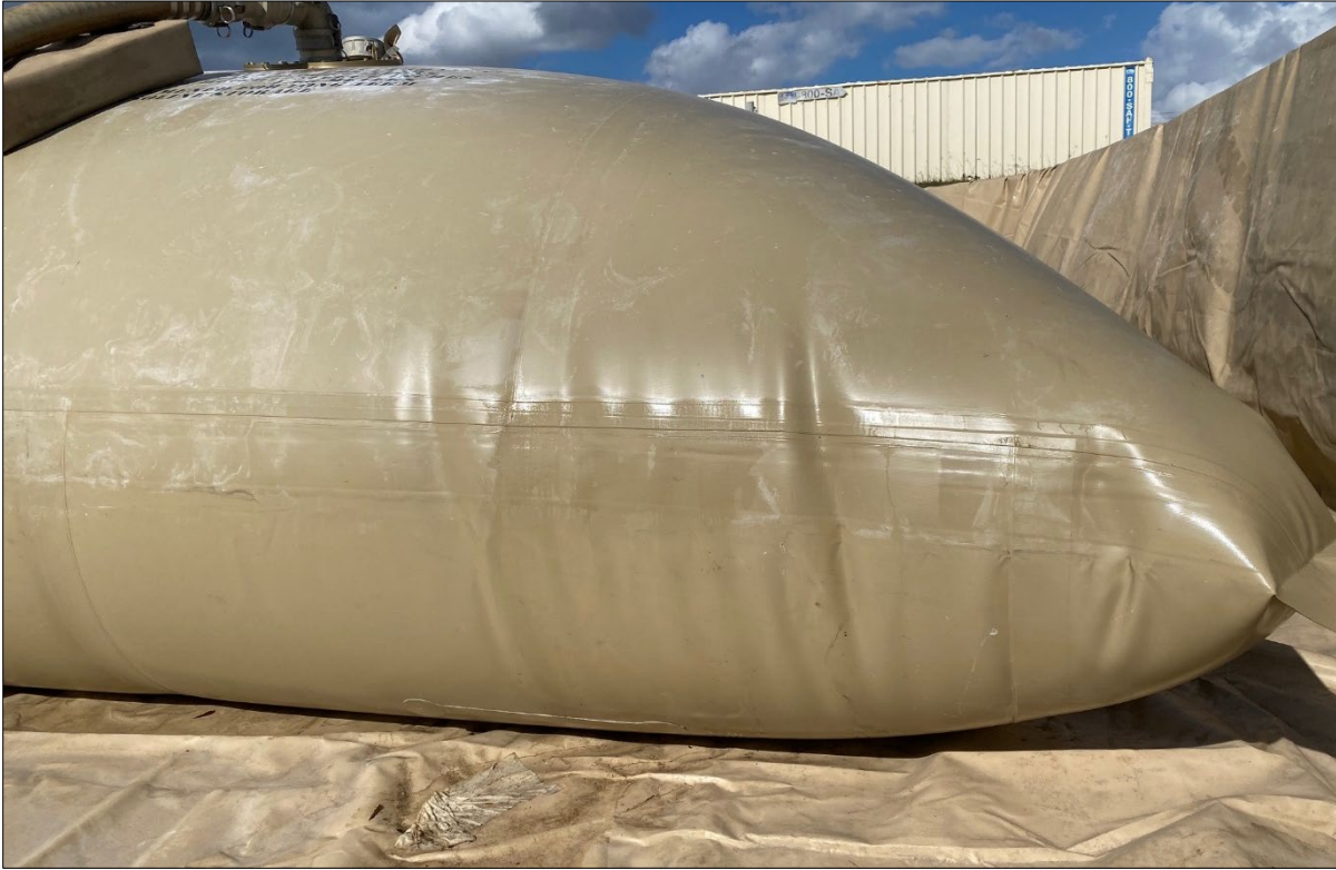
Figure D-3. MILPAWS #4 CFT Fuel Moistening at Seam
