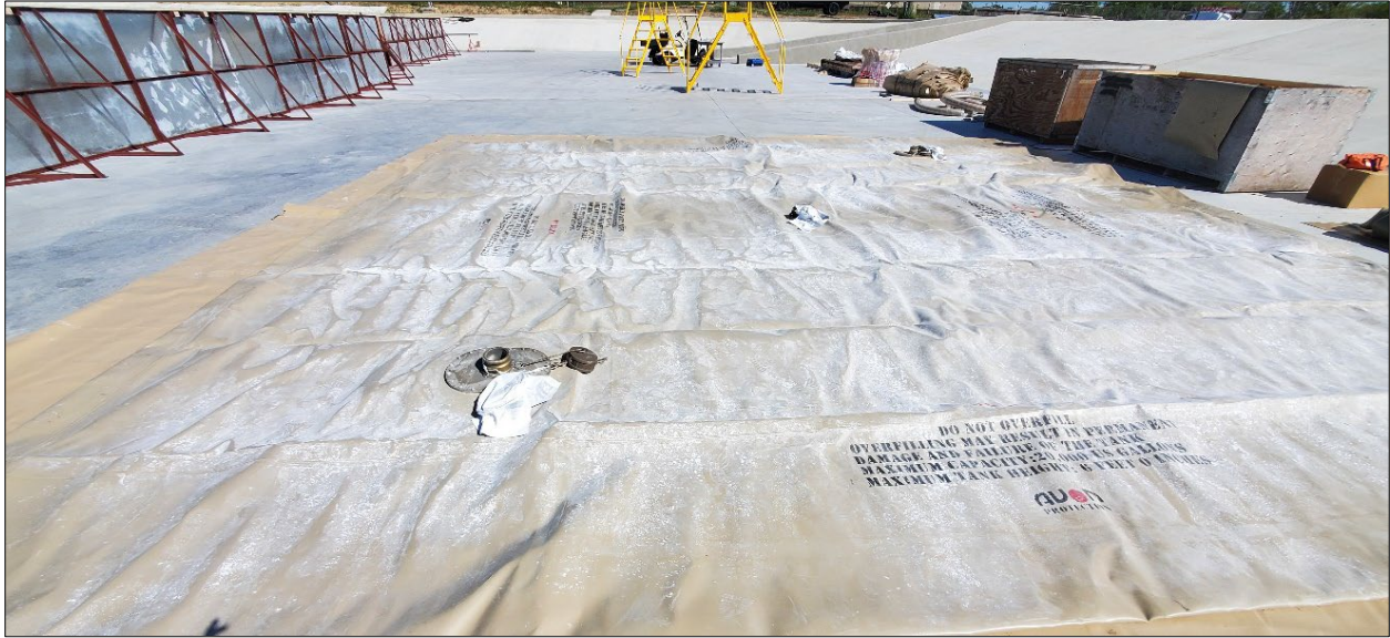
Figure C-2. AEF #3 CFT Unfolded and Deployed (Mfr. Applied Talcum Powder to Prevent Fabric from Sticking to Itself)
