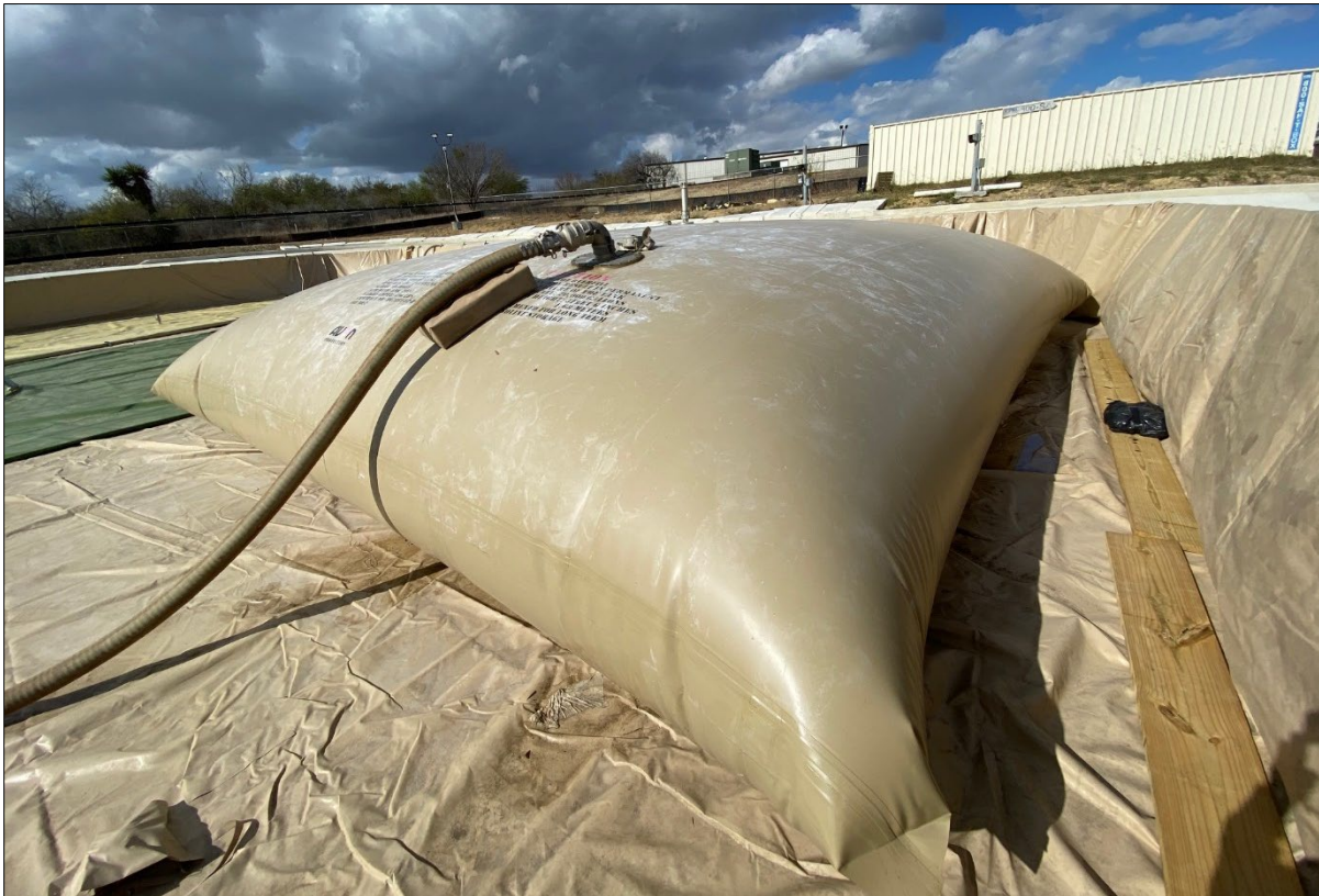
Figure D-2. MILPAWS #4 CFT Filled with Fuel
