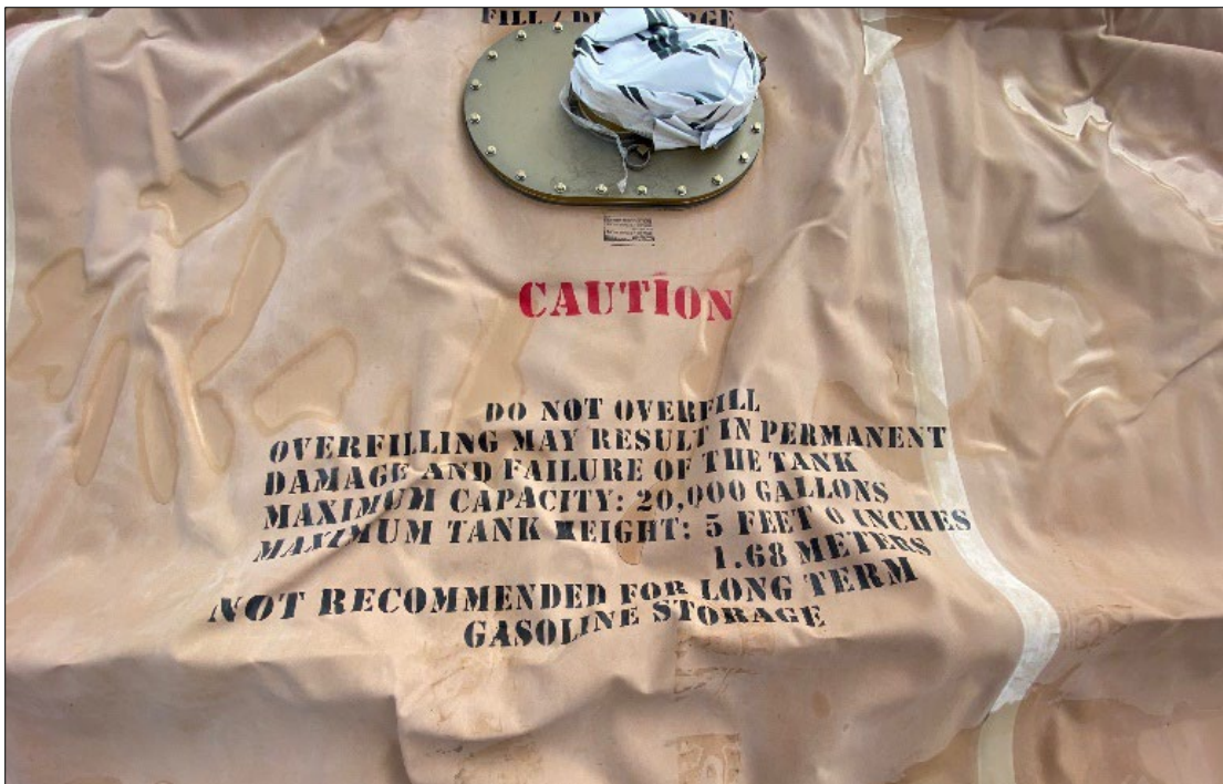
Figure B-2. JGB #2 NITRILE CFT Stencil on Tank Surface
