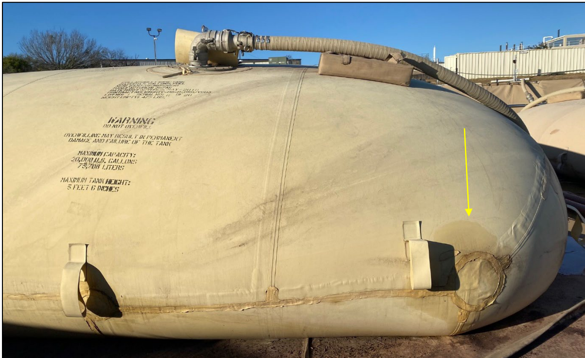
Figure F-5. MPC #6 CFT at End of Test Program, Showing Some Fuel Staining at Corner
