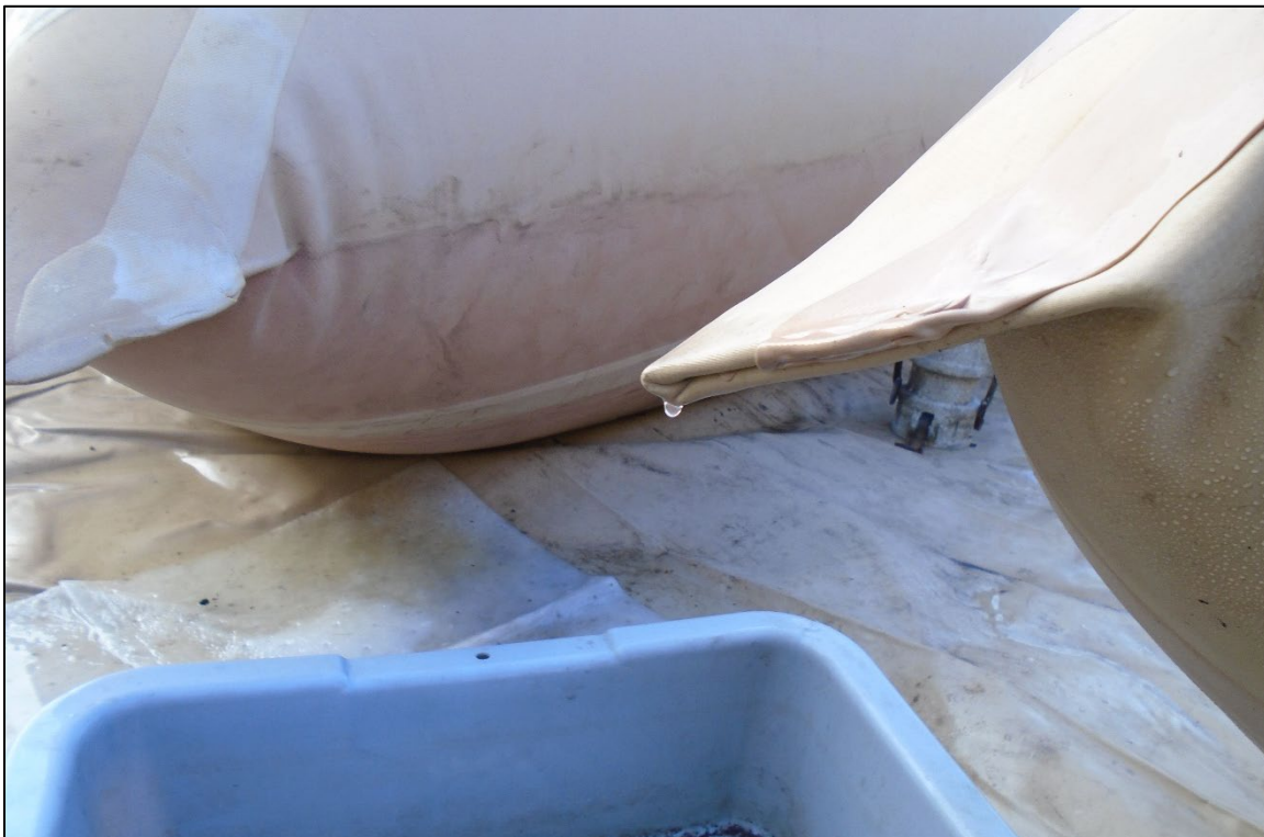
Figure E-6. AEF #5 CFT Fuel Drip Forming at Corner
