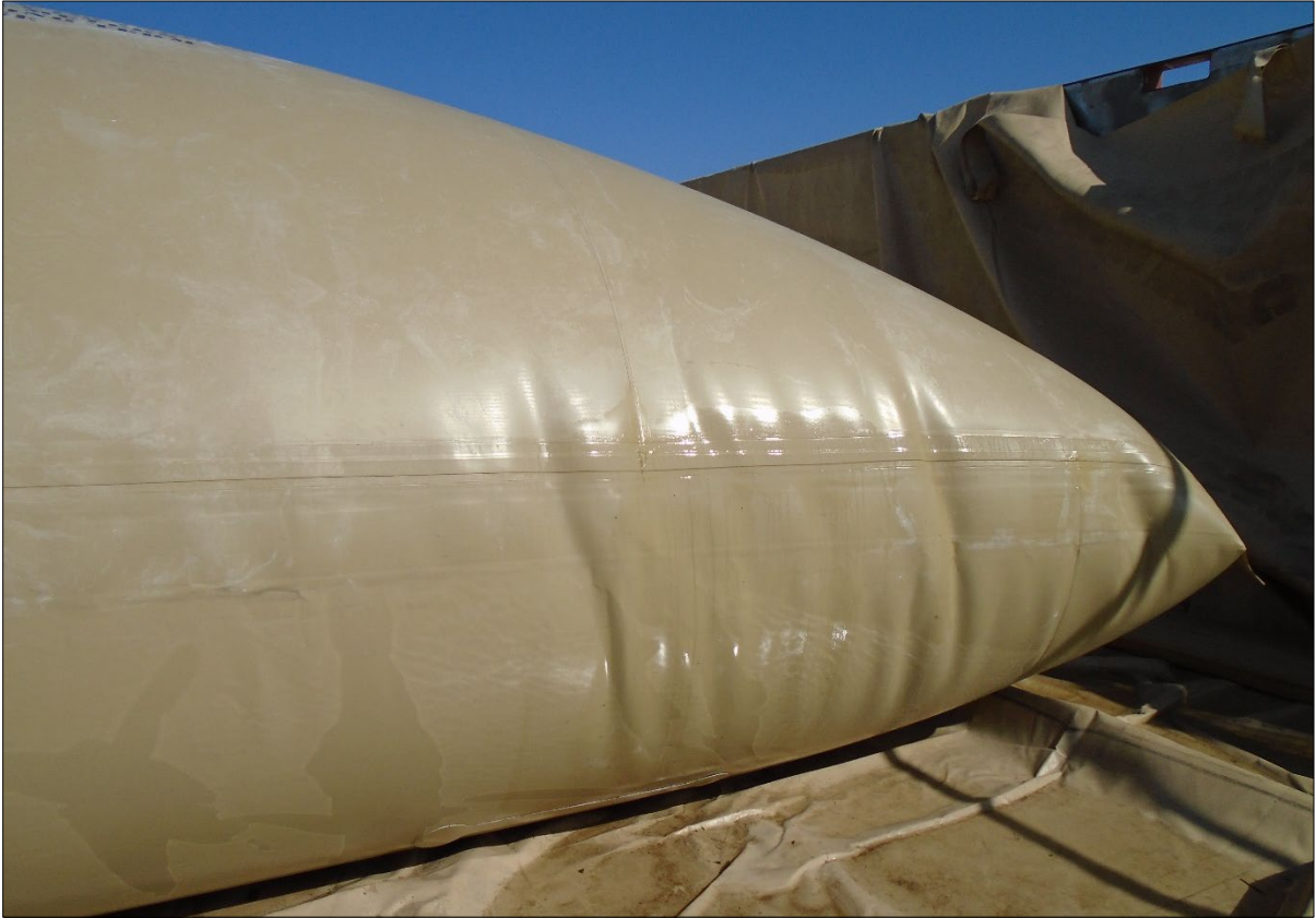
Figure D-7. MILPAWS #4 CFT Fuel Seeping from Seam
