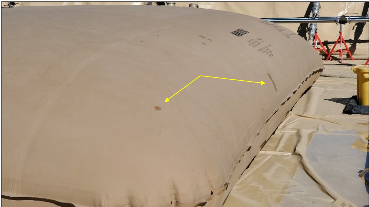
Figure A-4. BLSS #1 (NAFT #1) CFT with Fuel Leaks Through Fabric
