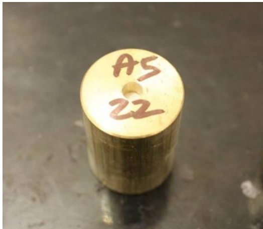
Figure 2 Picatinny Arsenal donor charge
