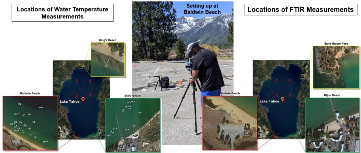
Figure 41 (left) Water temperature ground truth measurement locations (including RIT Tidbit data loggers in zoomed areas and JPL buoys as red “X” marks) and (right) RIT land temperature ground truth locations
