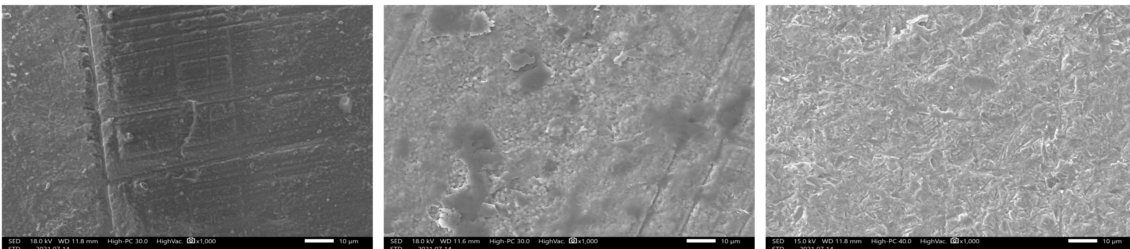
Figure 2. SEM Images (x1,000 / 10 μm) of STML with Various Surface Treatments. Left: No Air Abrasion; Middle: Air Abrasion with Glass Beads; Right: Air Abrasion with Aluminum Oxide.
