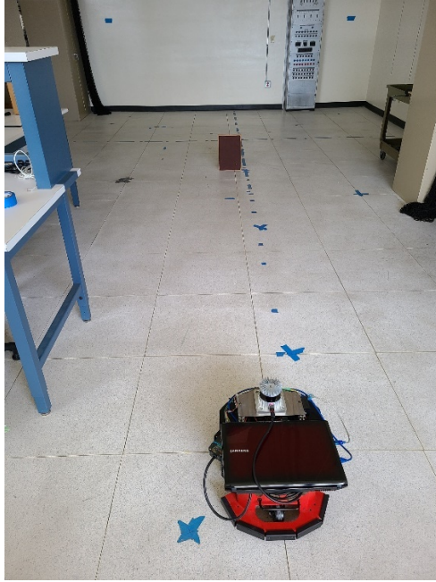
Figure 42. Experiment 1: Large Obstacle Detection and Avoidance
