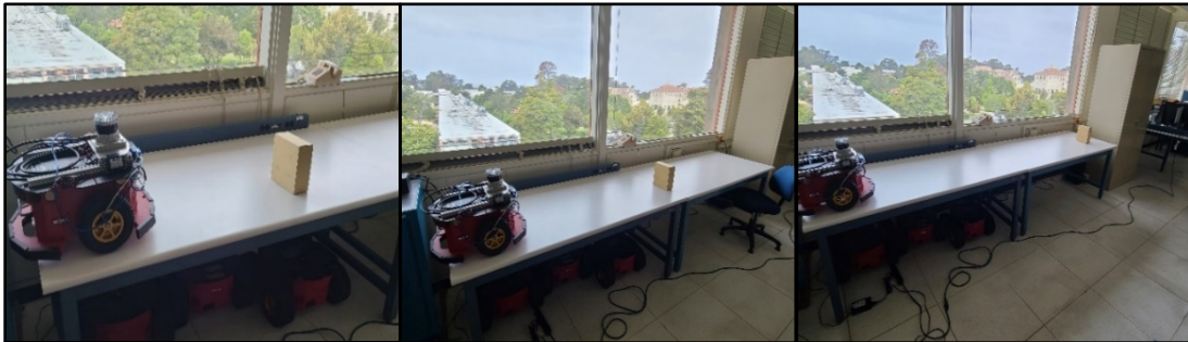
Figure 17. Small Object Test Setup at 0.8 m, 1.5 m, and 3.0 m
