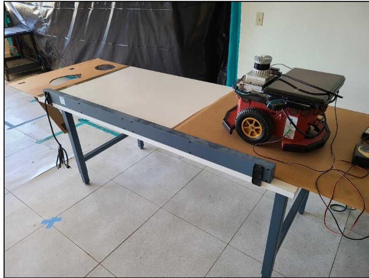
Figure 28. Negative Obstacle Detection Experimental Setup
