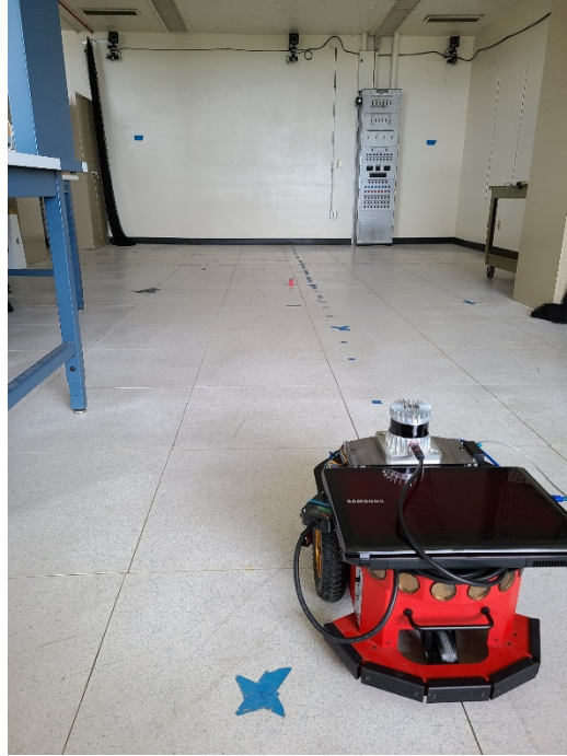
Figure 44. Experiment 2: Small Obstacle Detection and Avoidance
