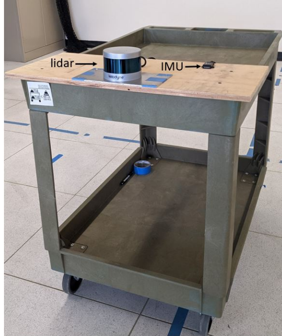
Figure 8. Cart with lidar and MicroStrain sensors
