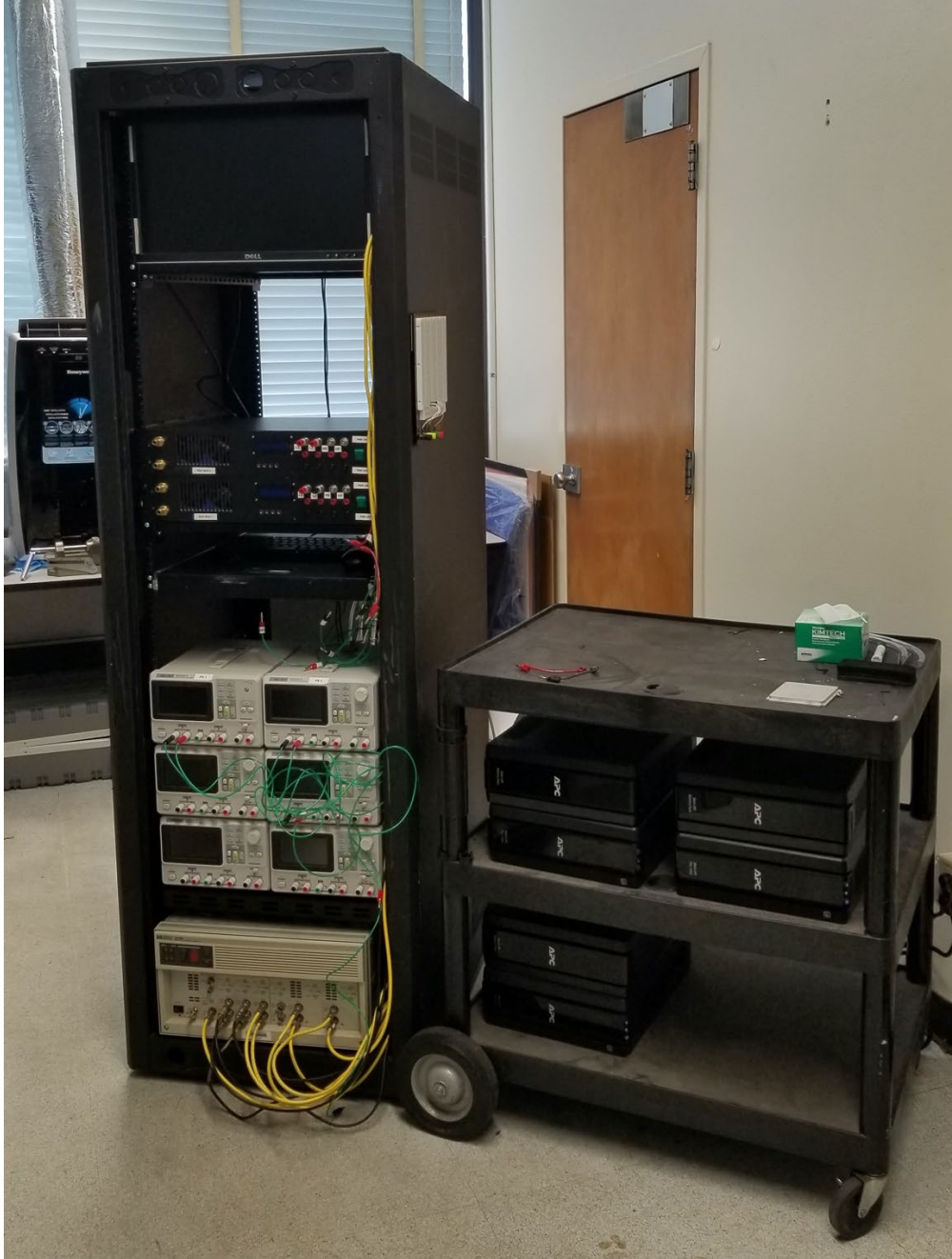
Figure 17. Image of constructed HTOL system with two stress test modules.
