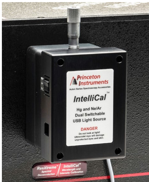
Figure 20. IntelliCal AE light source including Hg and Ne-Ar lamps. Source: [45].
