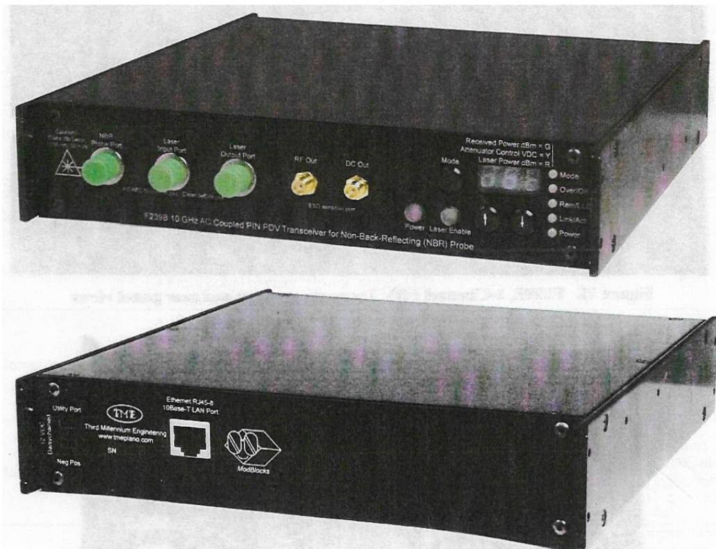
Figure 17. Front and rear view of Photonic Doppler Velocimeter (PDV) transceiver. Source: [43].
