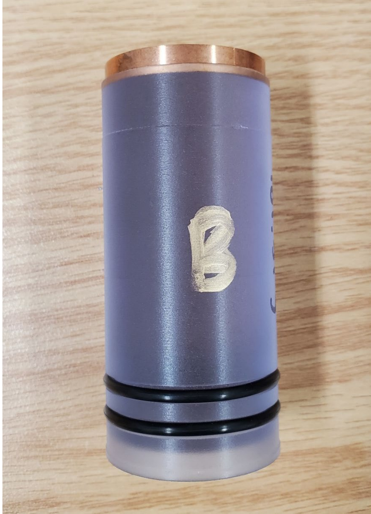
Figure 10. Fully assembled copper flyer-plate projectile, labeled "B."
