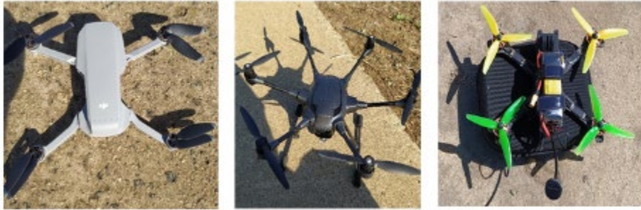
Figure 29. sUAVs with a maximum dimension of less than 60 cm used in the experiments.
