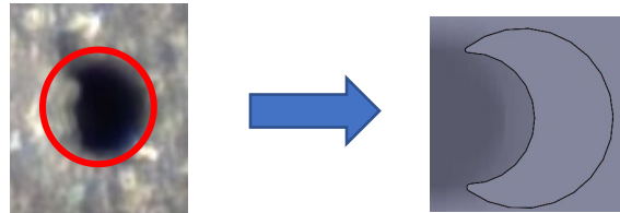
Figure 11. A close-up image of an injection site on an A15 injector block, and the injector shape used to simulate obstructed injection.
