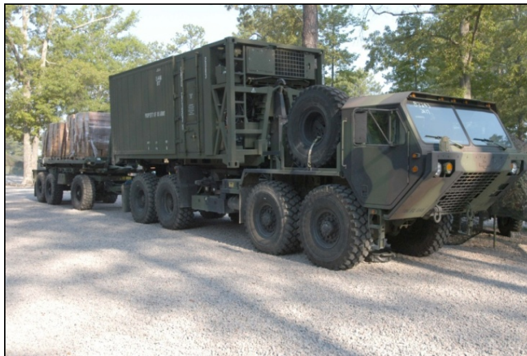
Figure 3. MTRCS and Flatrack on HEMTT-LHS and PLS Trailer. Source: ODASA (email to author, June 2011).
