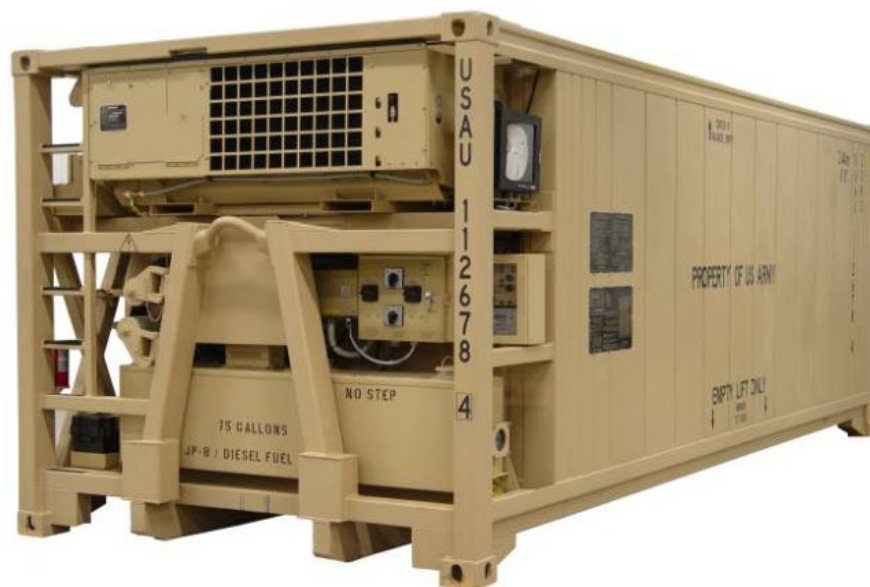
Figure 1. MTRCS Lifting End View Showing Integrated Bale Bar and Rail System Source: ODASA (email to author, June 2011)
