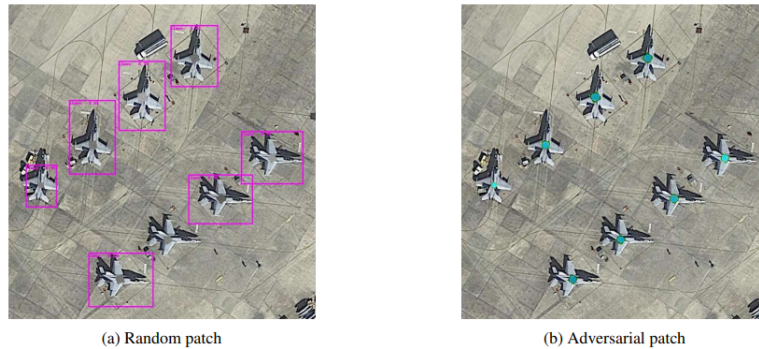
Figure 1.1. Images of aircraft with pink box overlays to indicate positive detection by detection algorithm. (a) Patches of random noise are overlaid on each aircraft image and shown to be generally unsuccessful at defeating the object detection algorithm. (b) Same aircraft but with adversarial patches causing no positive identification, thereby defeating the detection algorithm. Source: Adhikari et al. (2020).
