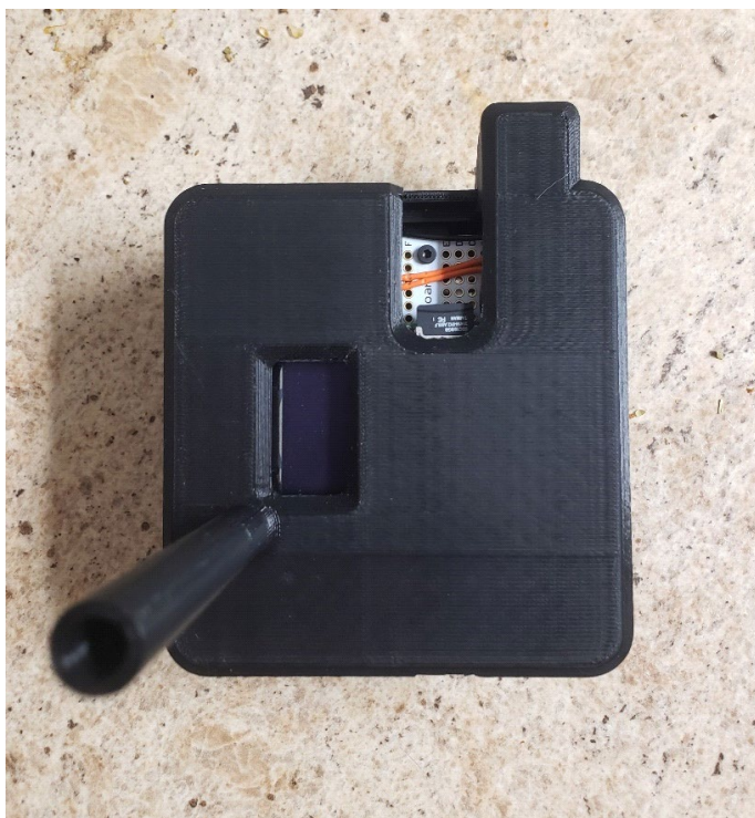
Figure 2: The exterior of the server
