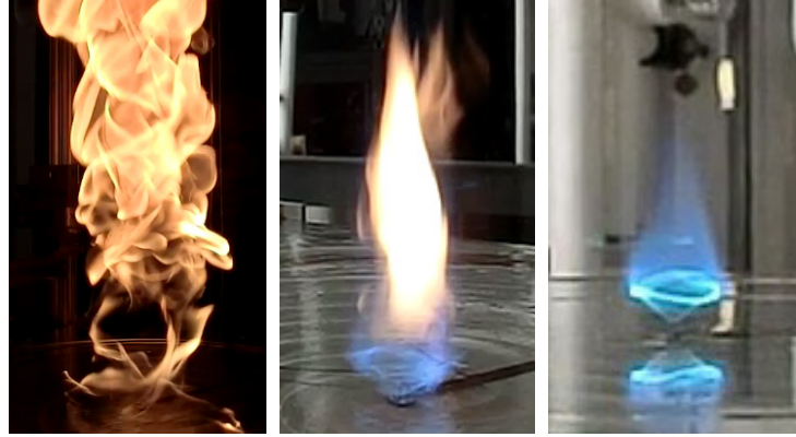
Fig. 1 The three stages of blue whirl formation: (left to right) fire whirl, transitional whirl, and blue whirl
