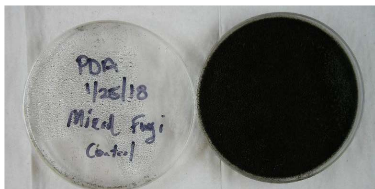
Figure 3. Potato dextrose agar 7 days after inoculation with mixed, five-specie fungal spore suspension. Growth on PDA confirmed fungal spores were delivered to panels surfaces.
