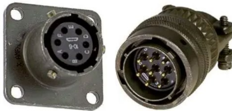
Part numbers are MS3112E10-6S and MS3116F10-6P.
