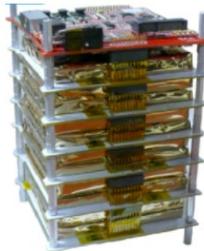
Figure 68. CubeSat battery matrix. Source: [28].
