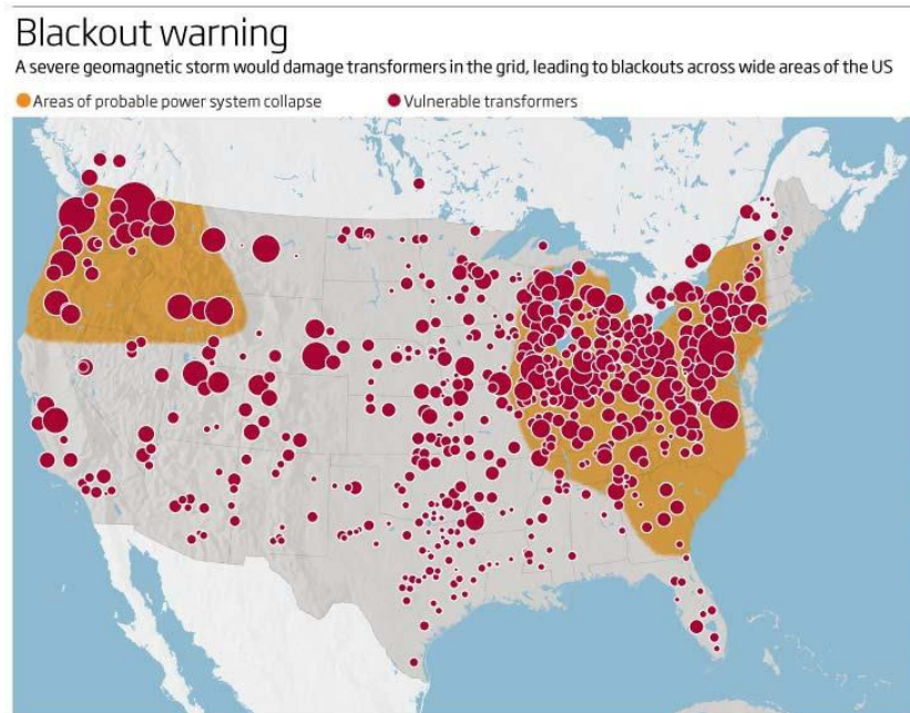
Figure 3. Map depicting transformers vulnerable to GICs (red) and possible blackouts due to transformer failure (yellow) 97
