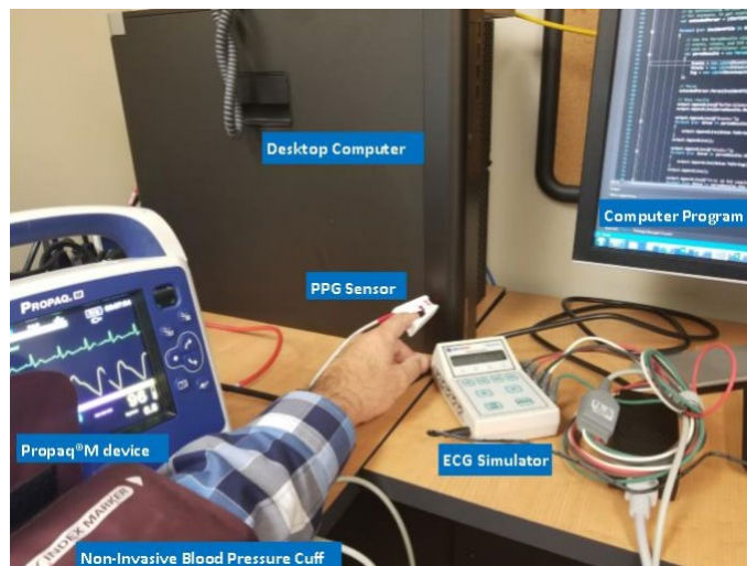
Figure 2. A demonstration of getting VS data from Propaq M device and process in a regular PC
