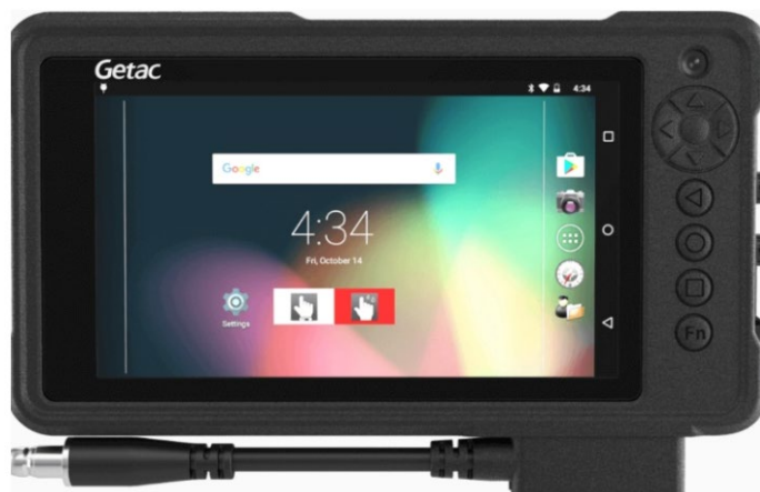
Figure 24. Rugged Android device that used for running the data acquisition software
