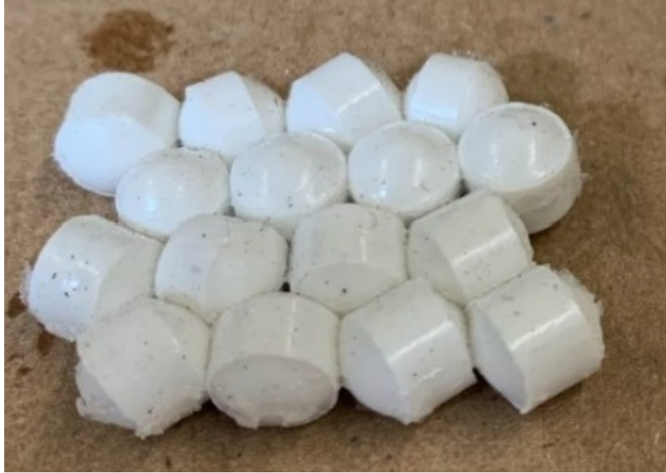
Figure 23. Sample target of AD90 1/4" ceramic spheres.
