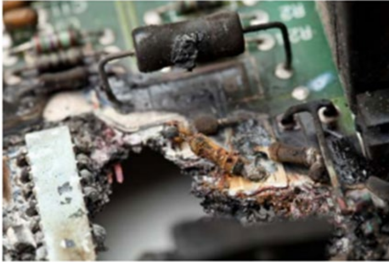
Figure 1. The Effects of a Low Level EMP Against Unshielded Electronic Circuits. Source: Mishra and Sashi (2014).
