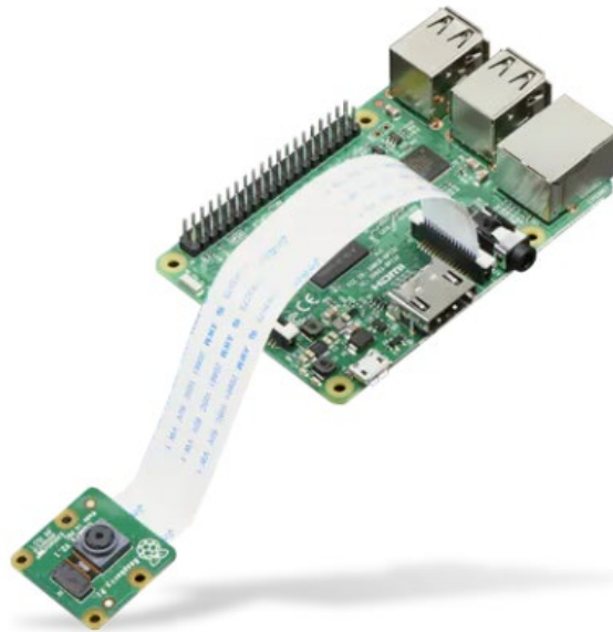
Figure 25. Raspberry Pi and V2 Camera. Adapted from [45].
