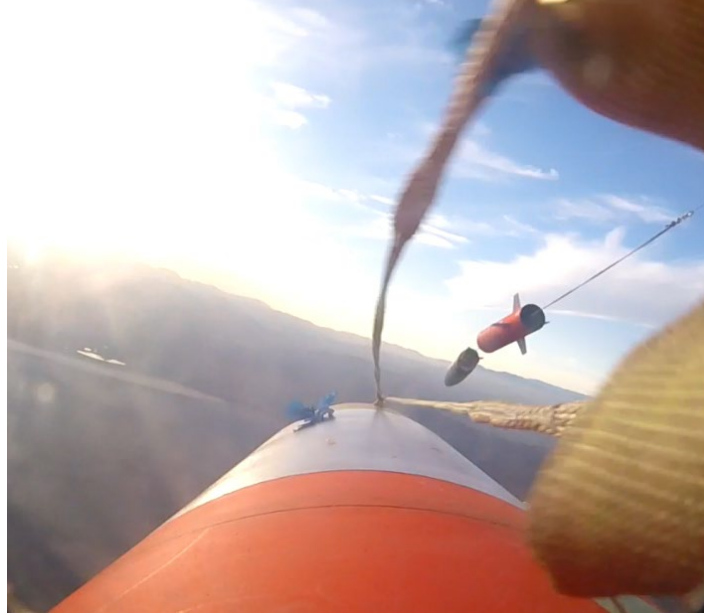
Figure 28. Premature Separation of Sled and Nosecone.
