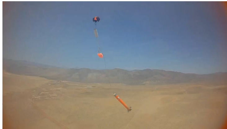
Figure 64. Nosecone Camera View of Booster Deploying Main Parachute.
