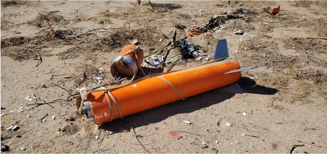
Figure 78. Rocket 5 Booster After Hard Landing.
