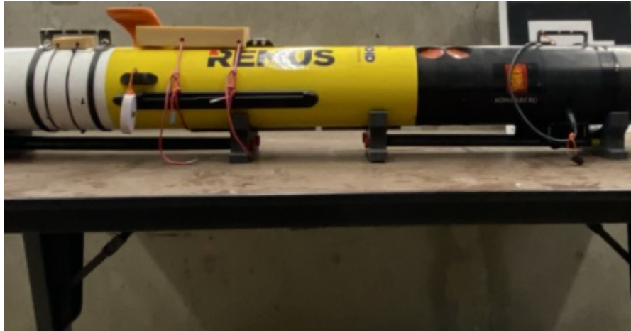
Figure 5.6. REMUS Outfitted With Flotation
