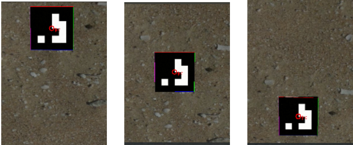
Three sequential seafloor AprilTag images demonstrating the AprilTag is entering and exiting the onboard camera's field of view. The AprilTag remains in the horizontal center of the field of view. The optimal image capture is when the AprilTag is in the center of the horizontal and vertical field of view.
