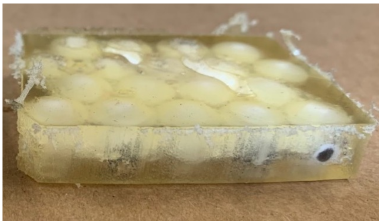
Figure 14. Versalink P1000 Encapsulate 3/8" Ceramic Spheres
