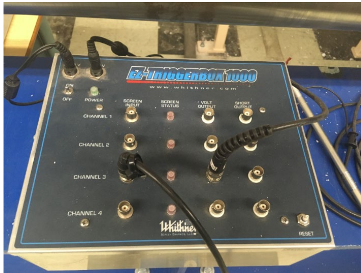
Figure 28. Whithner EZ-Triggerbox 1000. Source: [1].
