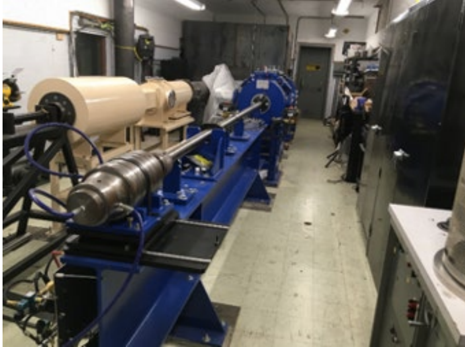
Figure 19. 1” Light Gas Gun. Source: [1].
