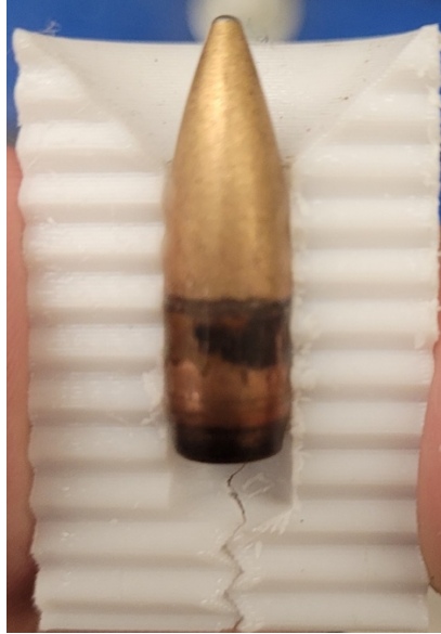
Figure 18. Cross-Section of Sabot with 7.62 x 39mm AK-47 Ball Projectile.
