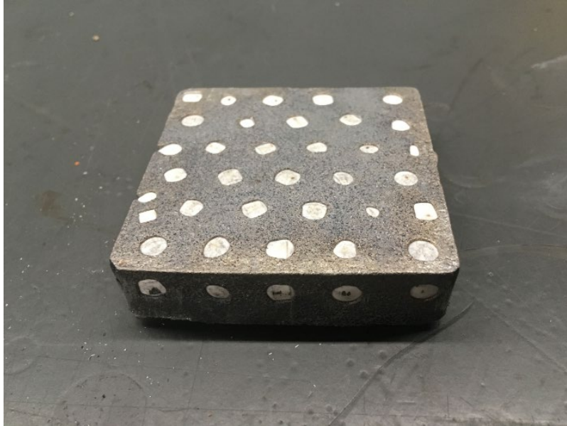
Figure 13. T6 Tempered A319 Aluminum Alloy Encapsulate 3/8" Ceramic Spheres
