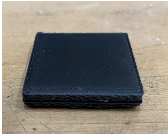
Figure 47. Carbon fiber-filled Nylon filament.
