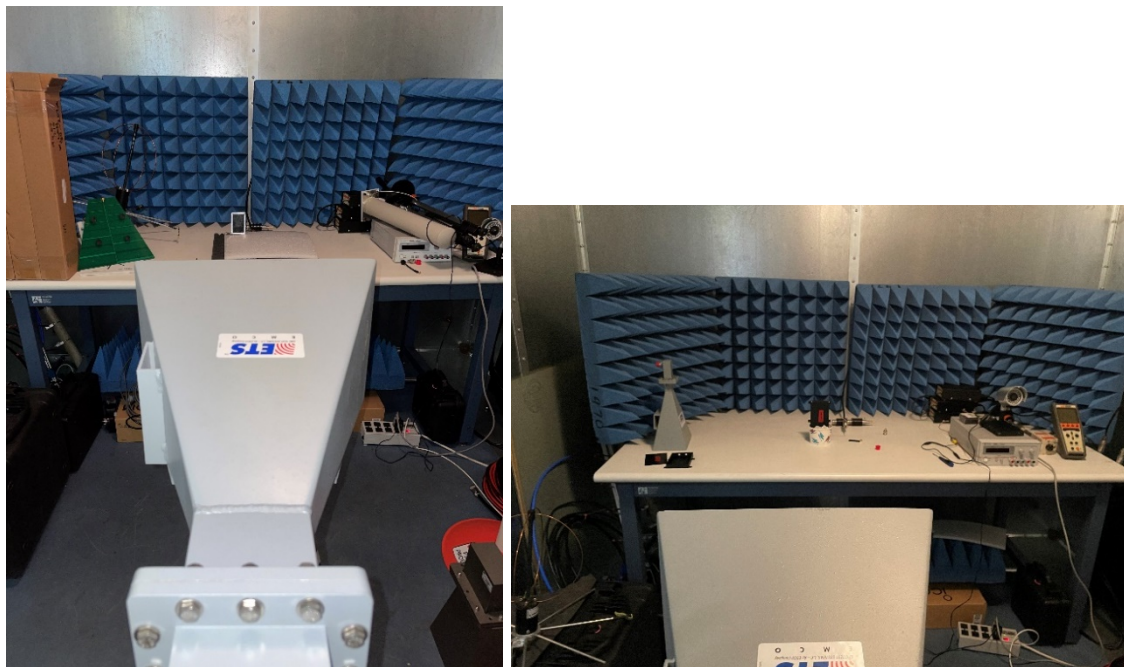
Figure 30. SE test setup with nylon (left) and ESD PETG (right).
