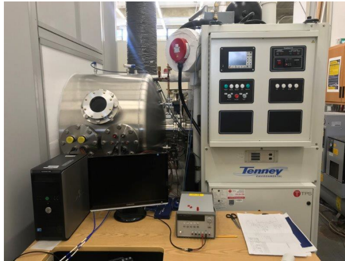
Figure 31. Tenney vacuum chamber. Source: [42].
