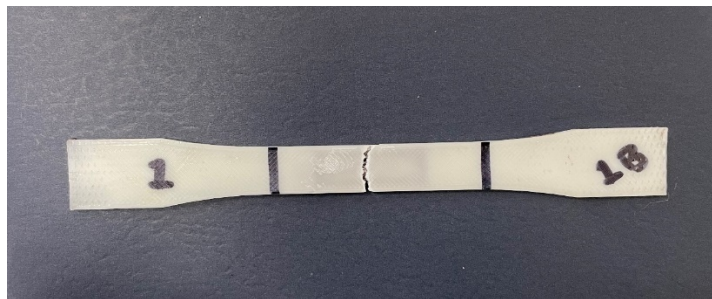
Figure 20. First of six test specimens after tensile testing.
