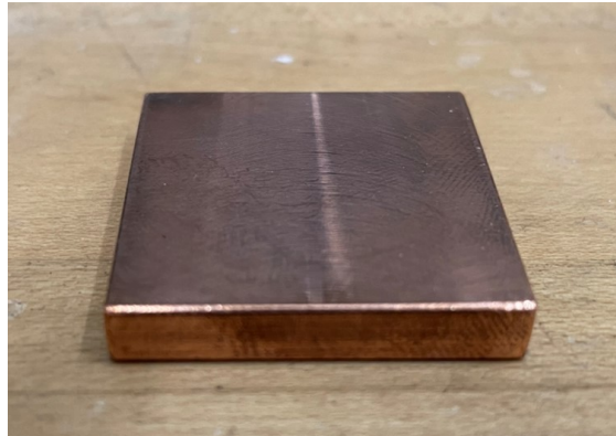
Figure 43. Solid Copper sample tested to validate the thermal conductivity test setup.
