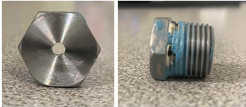
Figure 15. Fabricated 1/16" Exit Nozzle. Source: Reina [8].
