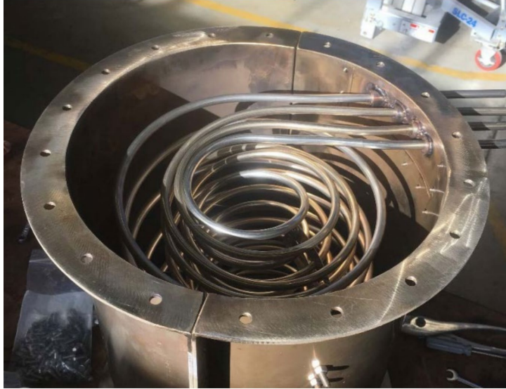
Figure 3. Heat Exchanger Coil Alignment. Source: Reina [8].
