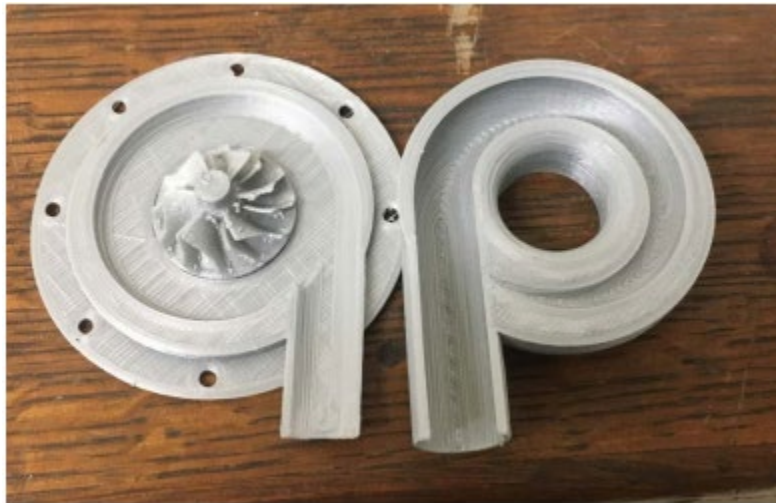
Figure 22. 3D Printed Volute. Source: Kaim [4].
