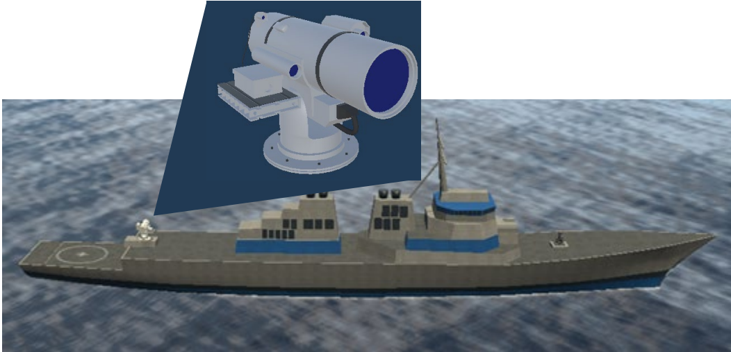
Figure 36. Surface vessel with LWS mounted aft. Adapted from Johnson (2021c; 2021d).
