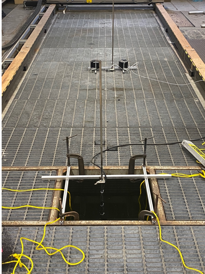
Figure 5. Geometry of the tow tank set-up
