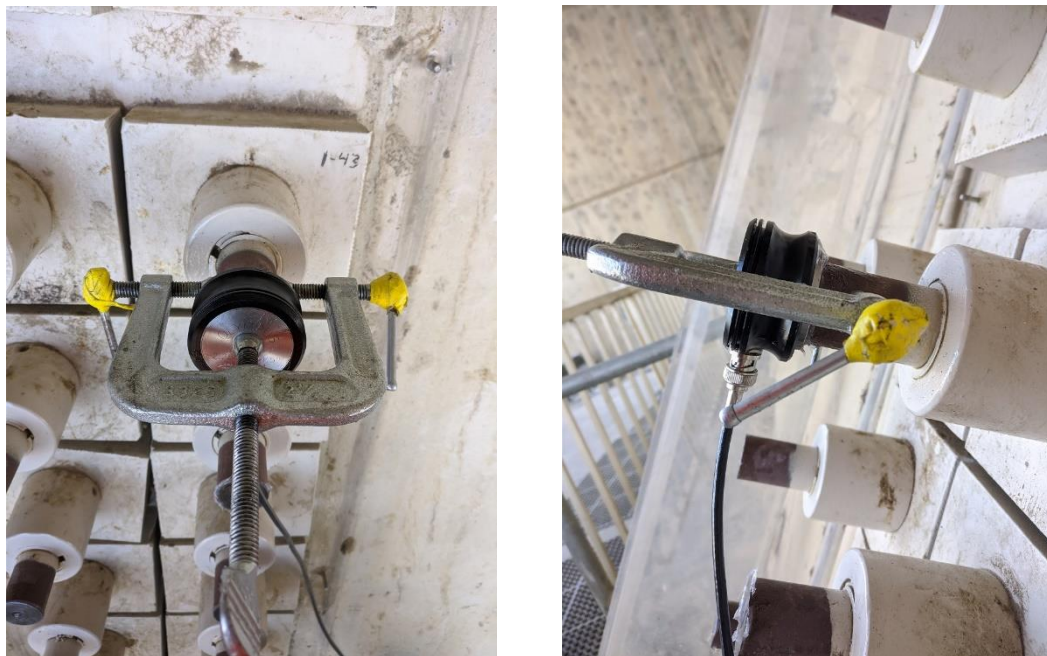
Figure 3. Transducer attached to tendon end.
