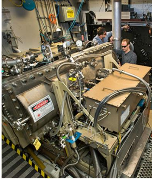
Figure 2 Photograph of the BNL CO 2 power amplifier [8] .
