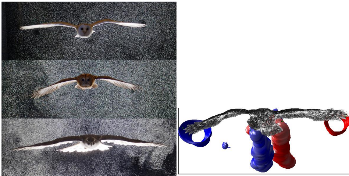
Figure 22 Wake visualization behind three birds demonstrates excess downwash behind the tail. Left) Multi-strobe-exposure photographs capture the wake behind a Barn Owl, Tawny Owl, and Northern Goshawk; top to bottom respectively. Right) Reconstructed wake of the Tawny Owl using Q -criterion to demonstrate the strong downwash induced behind the body and tail.
