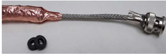
Fig. 12. The ferrite cores from Ferroxcube used and the gyromagnetic line built.
