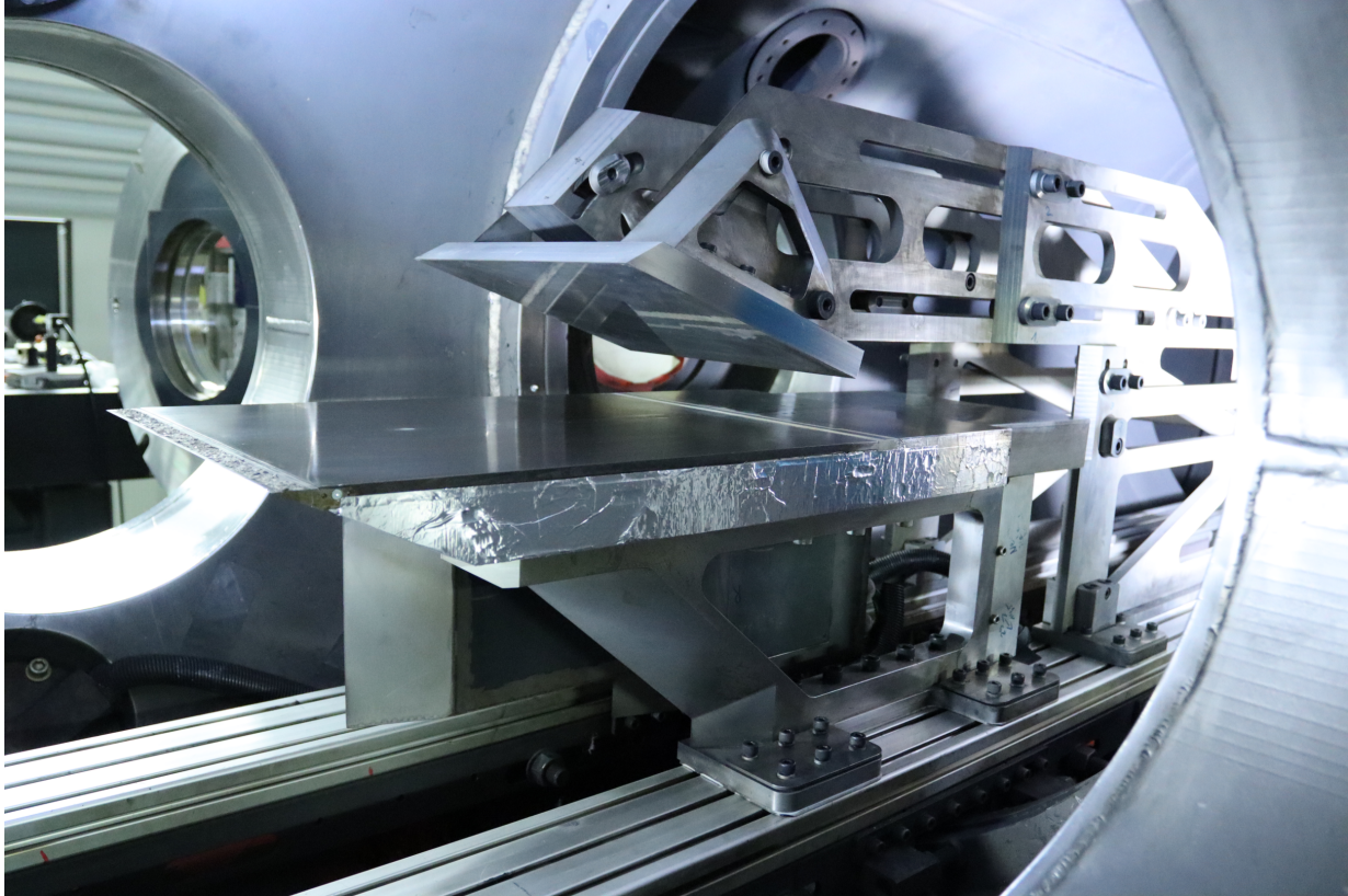
4-2 Flat plate and shock generator installed in the test section of the High Enthalpy Shock Tunnel Göttingen.
