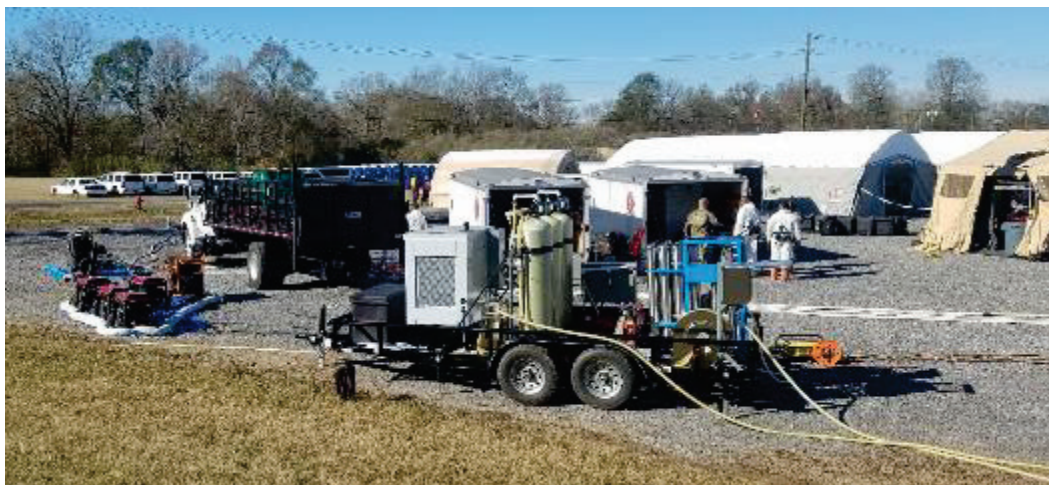
Figure 2. The Decontamination Effluent Treatment System (DETS).
