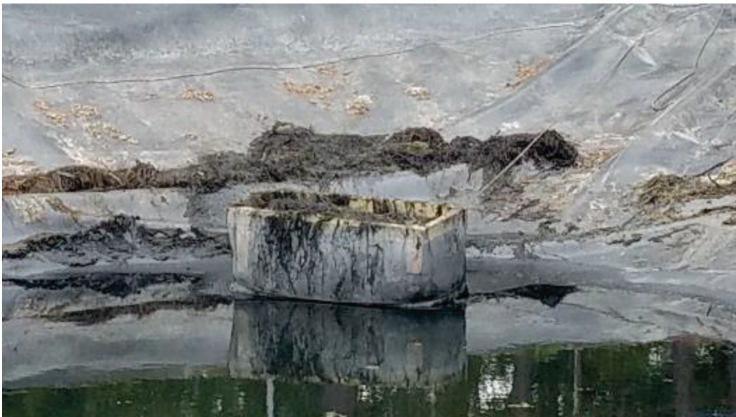
Figure 44. Filled sediment filtering box at end of demonstration 3.
