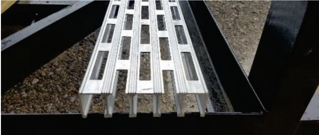
Figure 13. Aluminum planks installed on the PETS trailer.
