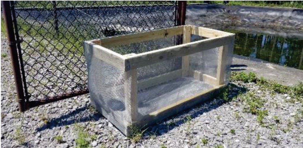
Figure 43. Screened box for sediment filtering.
