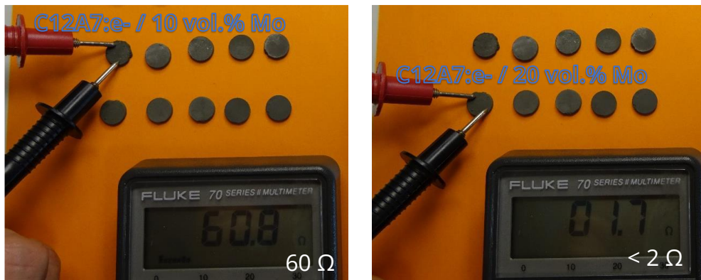
Figure 2.3-8 Rough measurement of the surface resistance by means of the probes of a digital multimeter. The resistance becomes smaller with rising molybdenum content.
