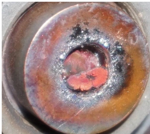
Figure 4.2-8 Red burnout residue from the insert, responsible for the electrical short to the keeper.
