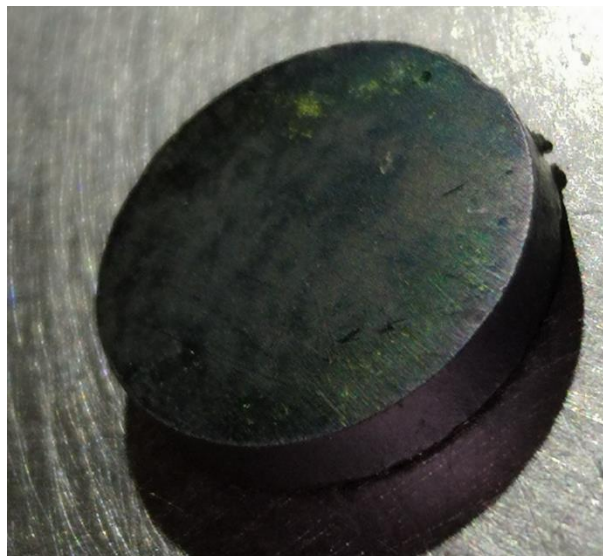
Figure 3.4-2 Specimen 3 after operation. Again, a metallic shine is detected and green areas are observed.
