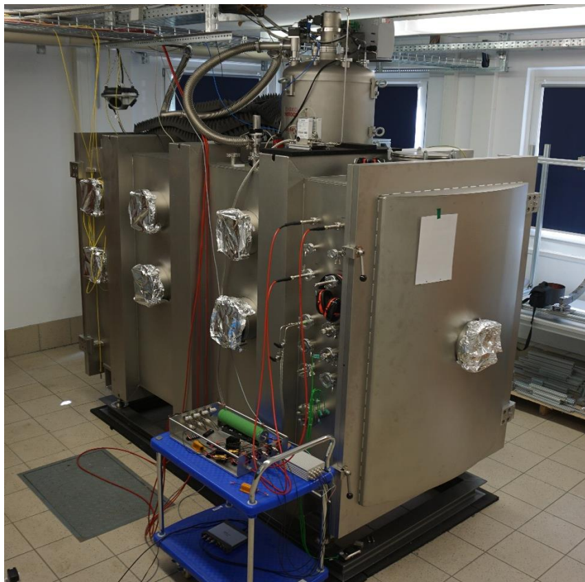
Figure 5.1-1 Vacuum chamber with electronics setup for endurance test.
