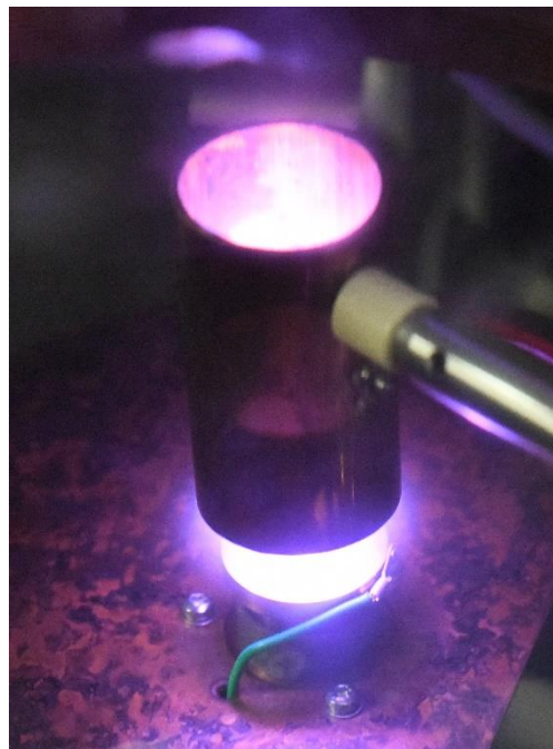
Figure 6.6-1 Operation of the C12A7 electride hollow cathode at one of the chambers at the Plasma and Space Propulsion Lab at UCLA.
