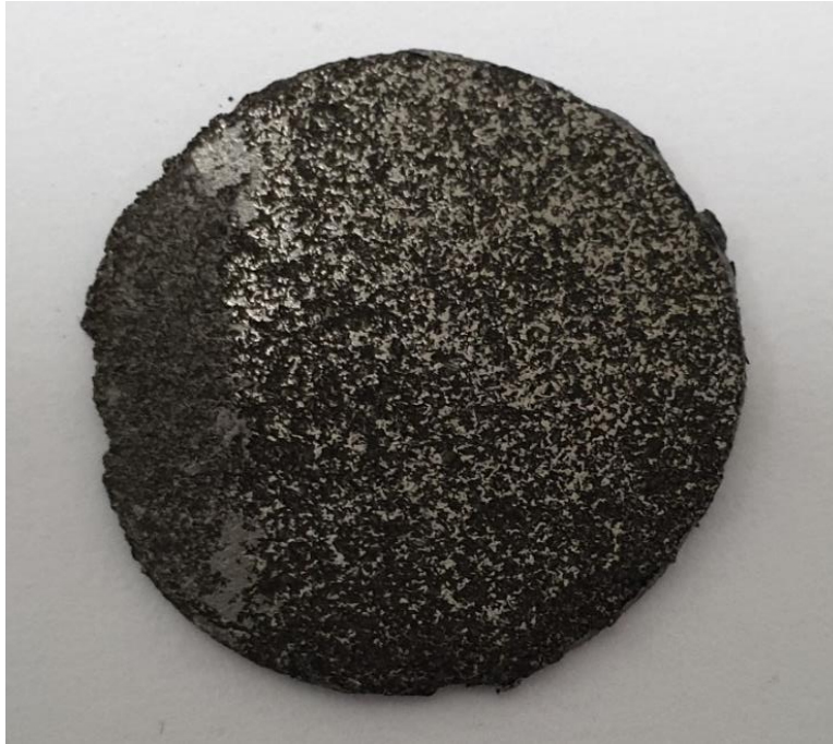
Figure 2.2-2 Sample with 30 vol.% of titanium. The diameter is 20 mm, the thickness 1 mm. The electrically conductive surface is very rough compared with the other samples
