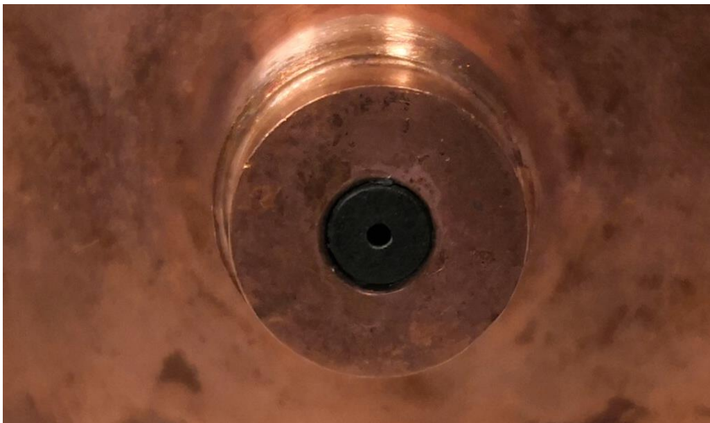
Figure 4.2-5 Fresh Insert in the Hollow Cathode setup AFRL_2.0. Insert is fitted tightly using electrically and thermally conducting carbon foil.
