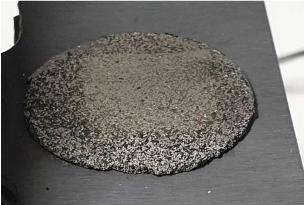
Figure 3.4-16 Titanium sample after thermionic emission test. Exposed / Emitting area can be seen clearly.
