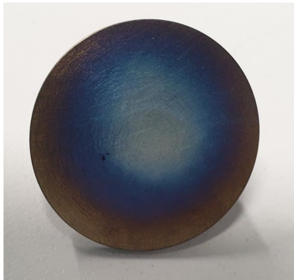
Figure 3.4-12 Picture of the front side of the anode (faced towards the specimen) after the test run at 1025°C/942°C.
