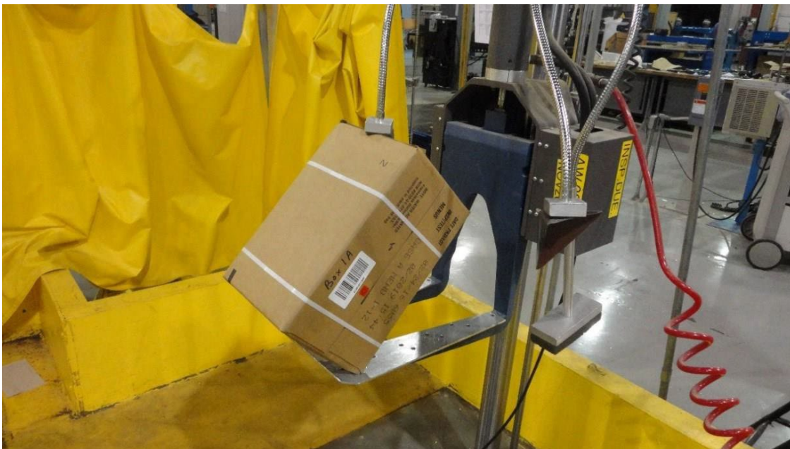
Figure 16. Free Fall Drop Test from 30 inches
