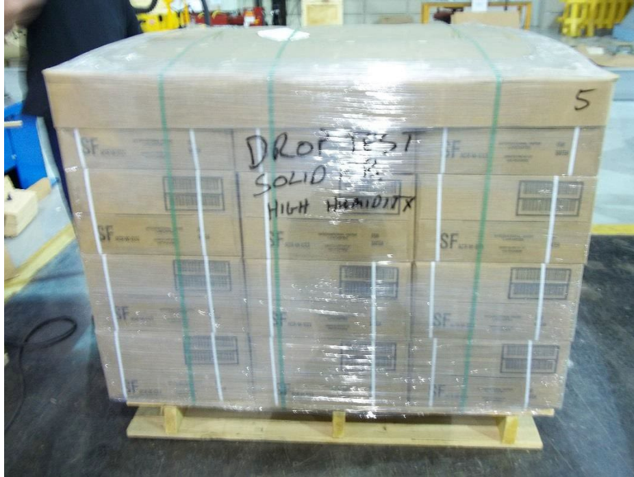
Figure 91. Solid Fiberboard Unitized Load (High Humidity Conditions) Following Rotational Drop Tests
