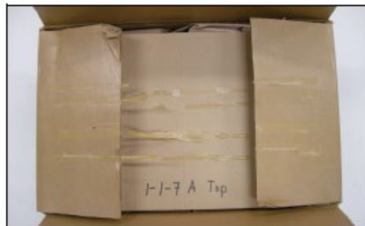
Figure 127. Adhesive failure on the top flaps during the assembly trial run
