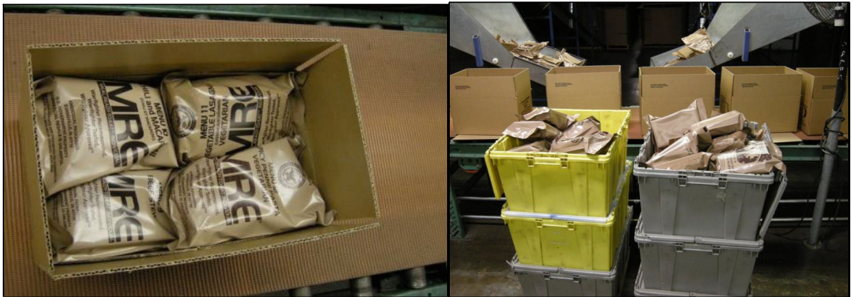
Figure 59. AmeriQual Packaging assembly line (left) and MRE filling station (right)
