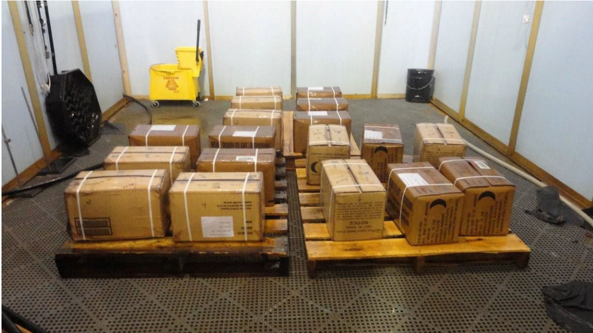
Figure 19. MREs Under Rain Test
