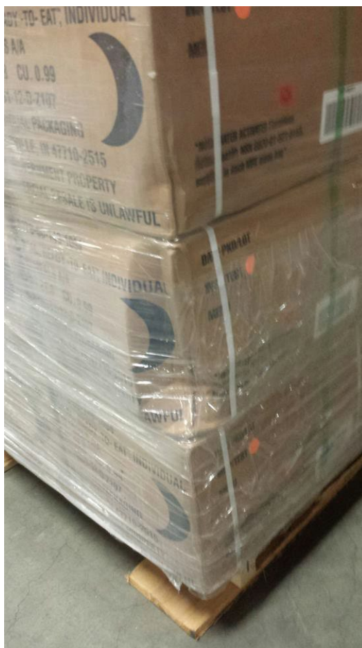
Figure 103. Large dent on edge of case on pallet
