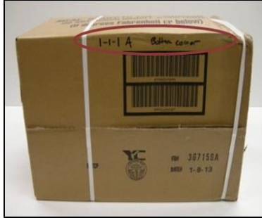
Figure 33. Bottom Crush. Stress creasing on bottom face of case, or creasing seen near the bottom edge.
