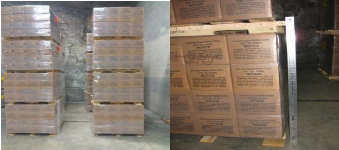
Figure 76. Pallets at Marengo Caves (left) and the deflection measurement system (right)
