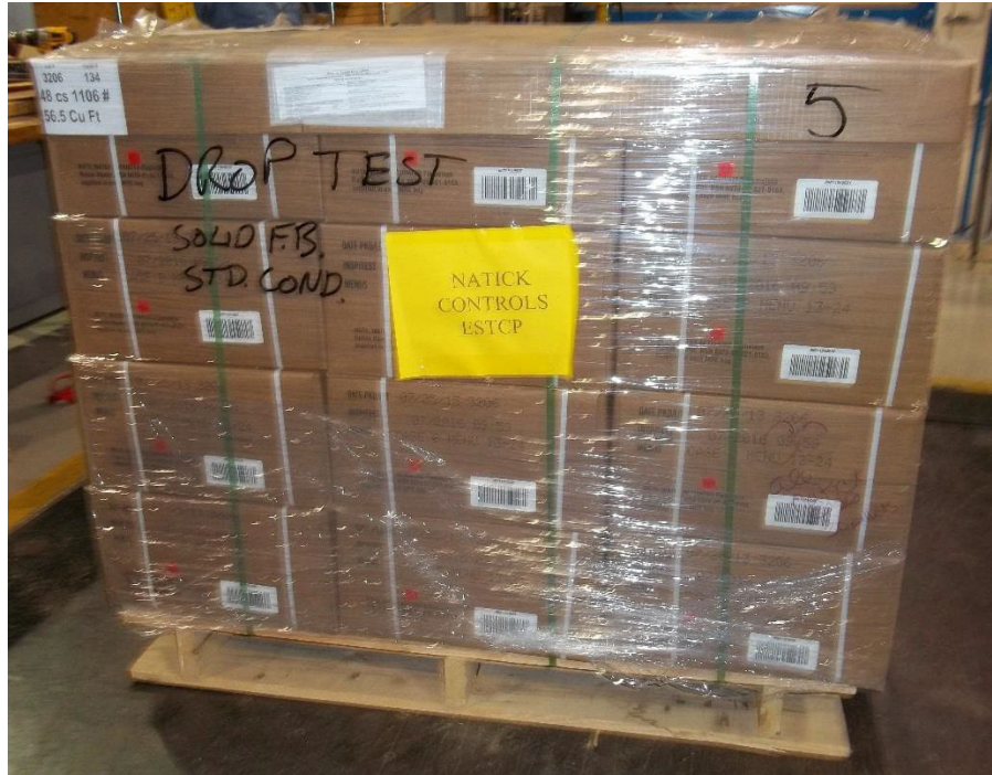
Figure 89. Solid Fiberboard Unitized Load (Standard Conditions) Following Rotational Drop Tests
