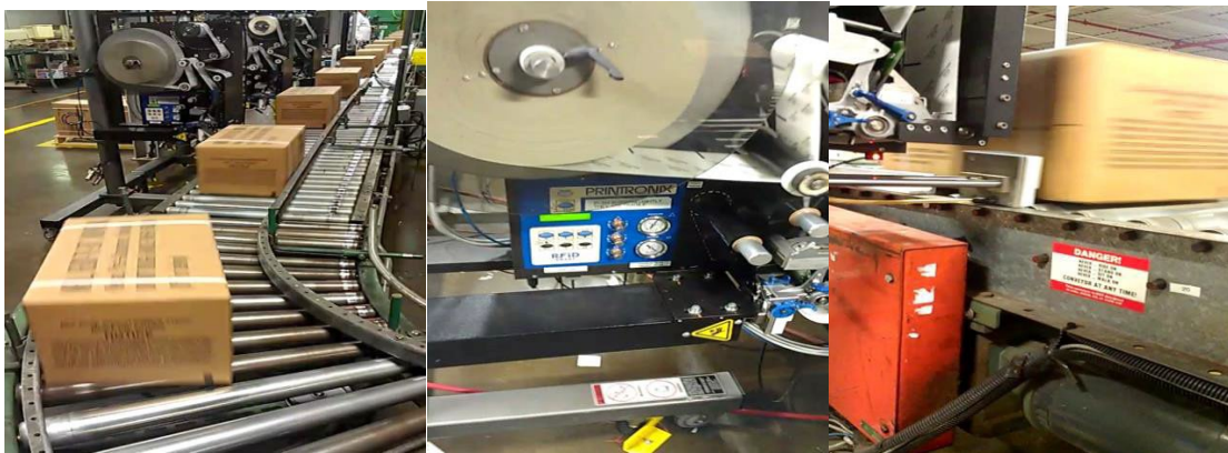
Figure 67. Labeling operations (left), barcode labeler (middle) and application of barcode (right)
