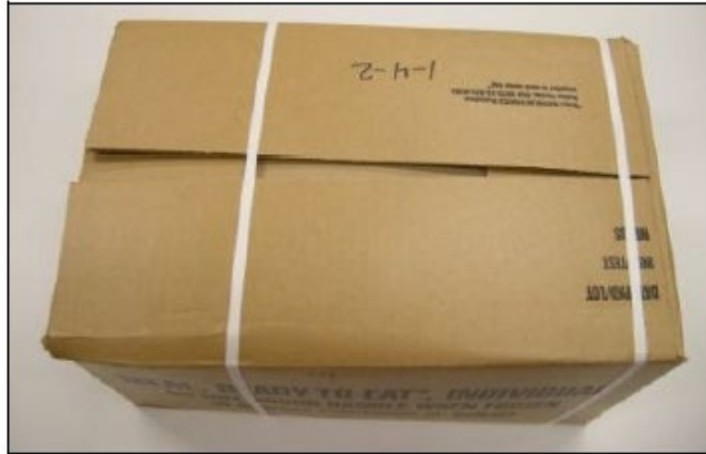
Figure 120. Excessive gap width of \frac{3}{4} inch or greater between the major flaps, normally caused by over-packing
