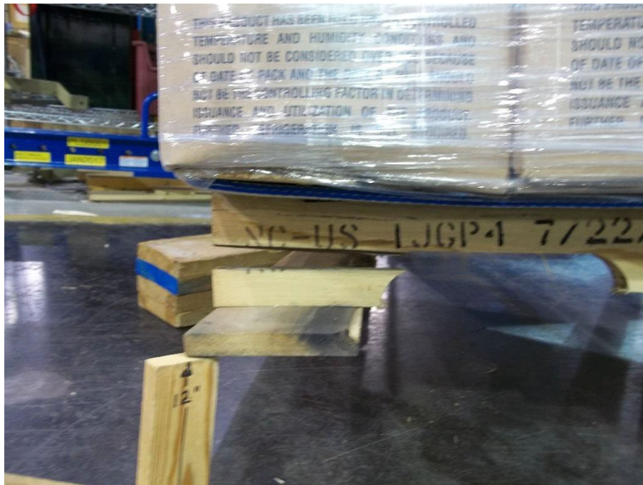
Figure 92. Cracked Stringer During Rotational Drop Tests
