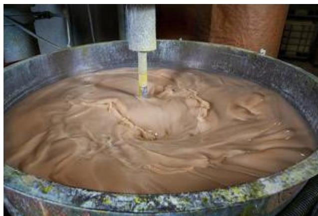
Figure 50. Blending the coating formulation
