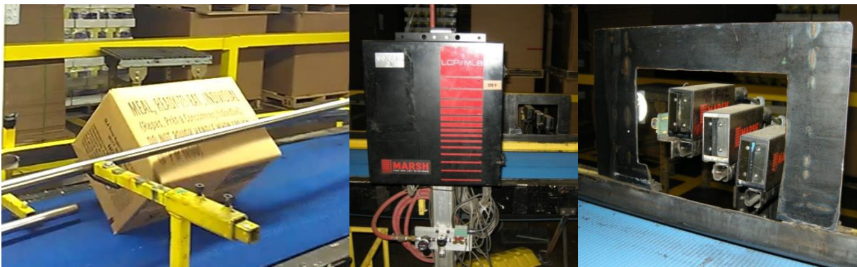
Figure 63. Orientation of case prior to print (left), Marsh LCP/ML8 printing station (middle) and three print heads (right) used to print the date of pack, inspection test date and case identification
