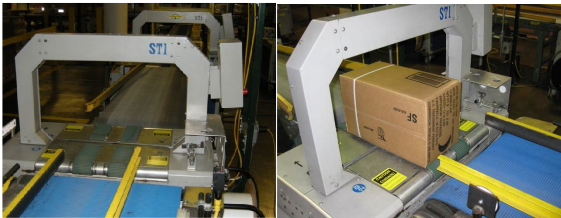
Figure 65. Case Strapping equipment used to band individual cases (left) and the strapped case (right)
