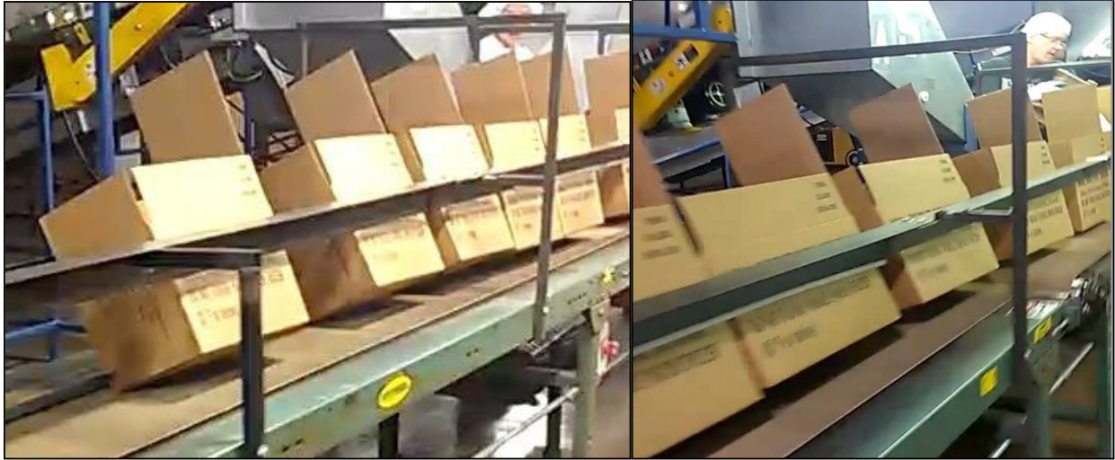
Figure 58. Fixed rail used to angle the cases towards line workers (left); rail tilted towards employee at filling station improving ergonomics and case packing activities (right)
