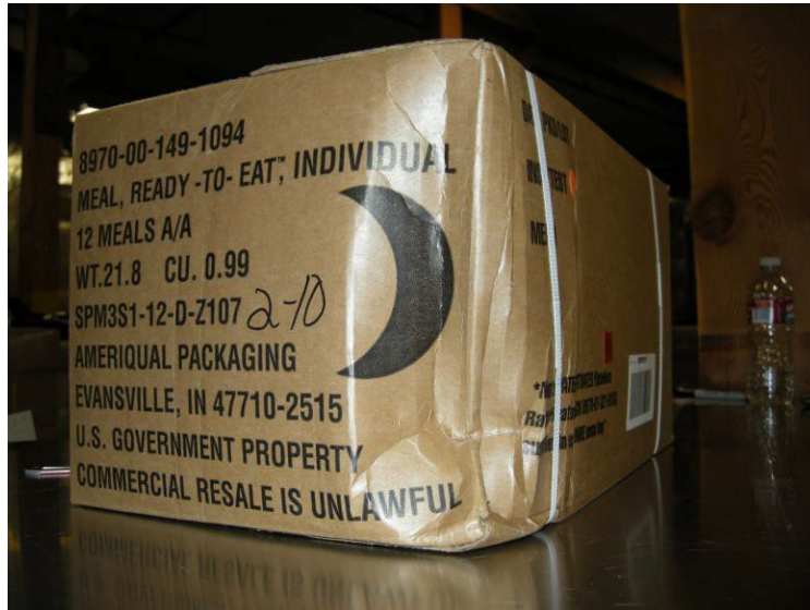
Figure 135. Dents on Pallet #1 Layer 2 Case 10
