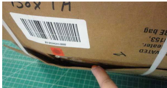
Figure 85. Glue separation on Solid Fiberboard
