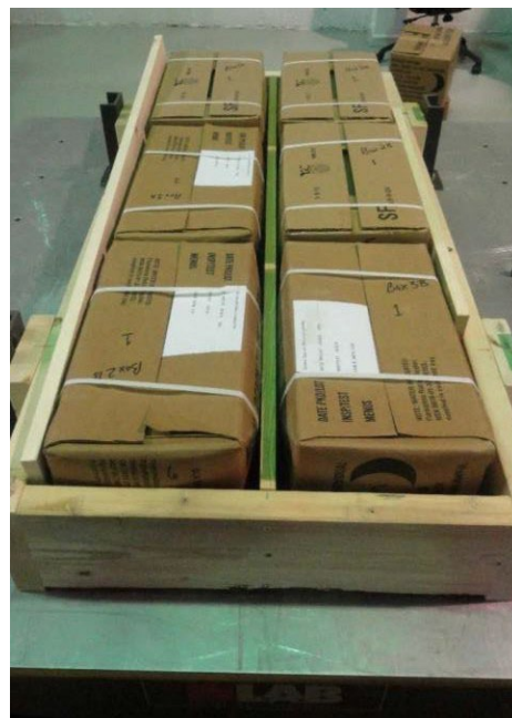
Figure 23. MREs during Random Vibration
