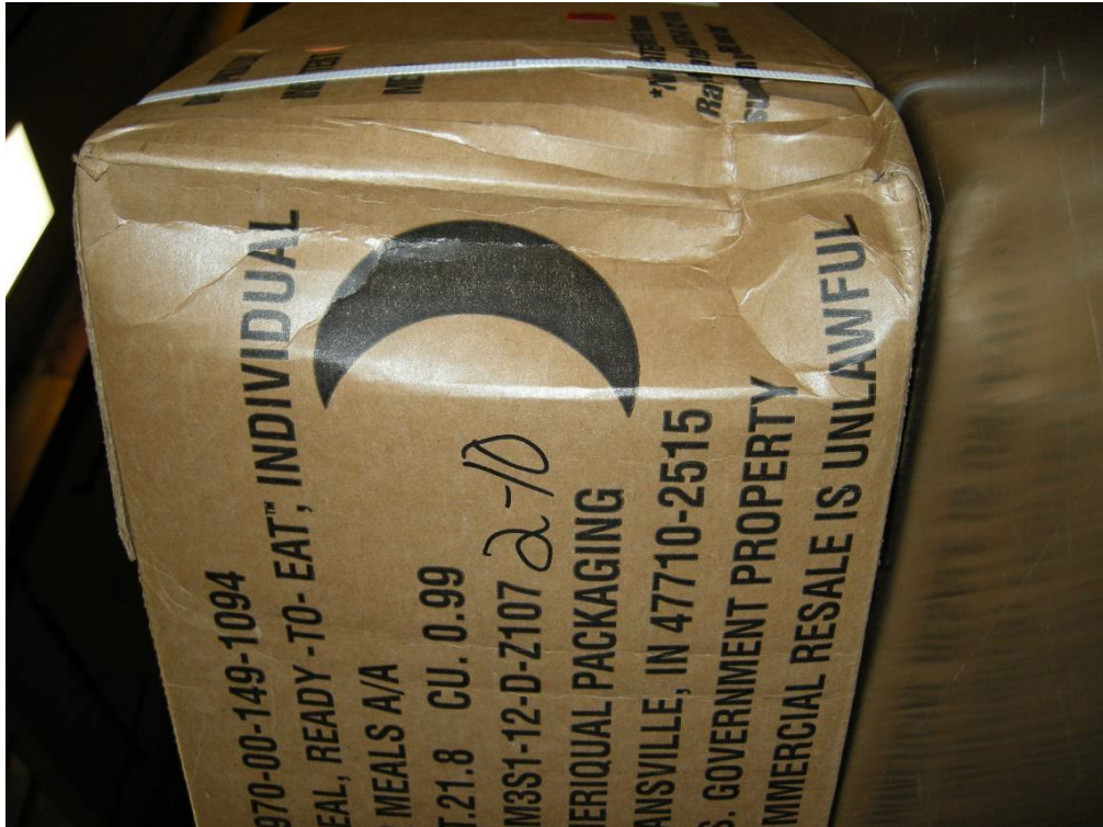
Figure 134. Damage to Pallet #1 Layer 2 Case 10
