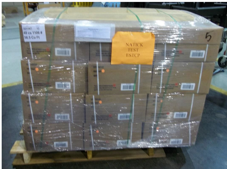
Figure 90. Corrugated Fiberboard Unitized Load (High Humidity Conditions) Following Rotational Drop Tests
