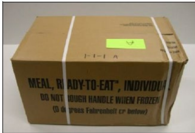
Figure 121. Crushing of the corrugated case during transit and or during material handling, pallet overhang was the primary cause of this type of damage
