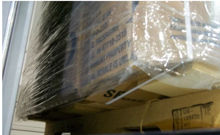
Figure 86. Corrugated Fiberboard Case Deformation (High Humidity Conditions)
