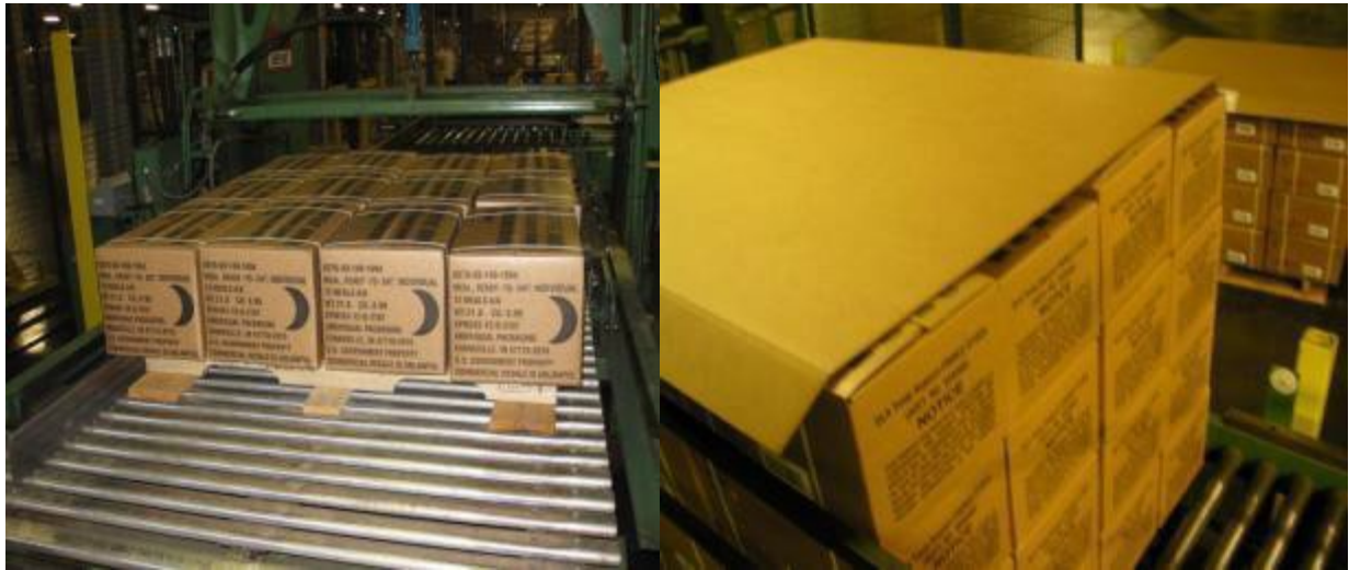
Figure 73. First level of cases in the palletizer (left) and the problem identified with the location of the cap folds on pallets of new cases (right)
