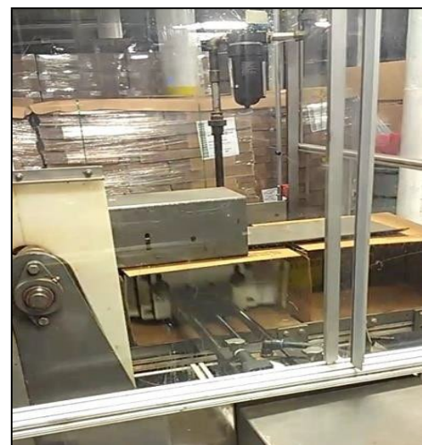
Figure 56. Full view of the case erecting equipment from Pearson Packaging Systems (left) and close up of the gluing of the case's bottom flaps (right)
