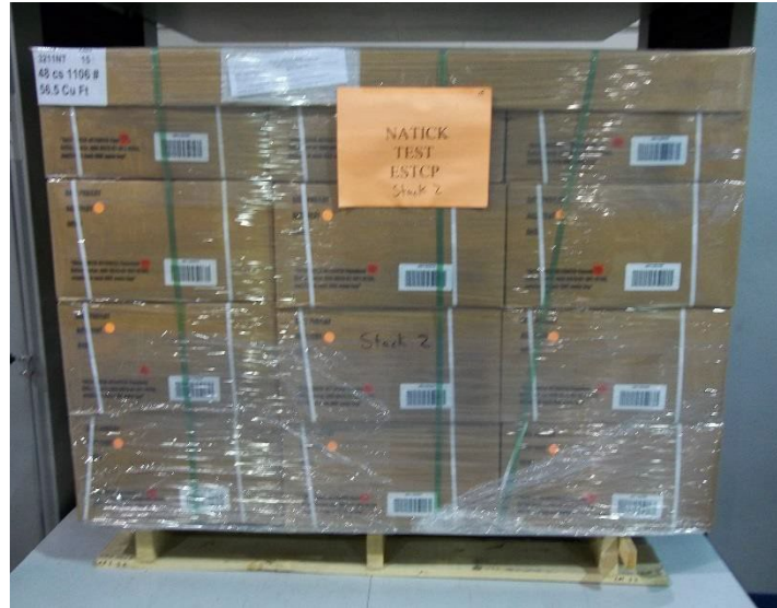
Figure 10. Compression Test of Corrugated Fiberboard Cases
