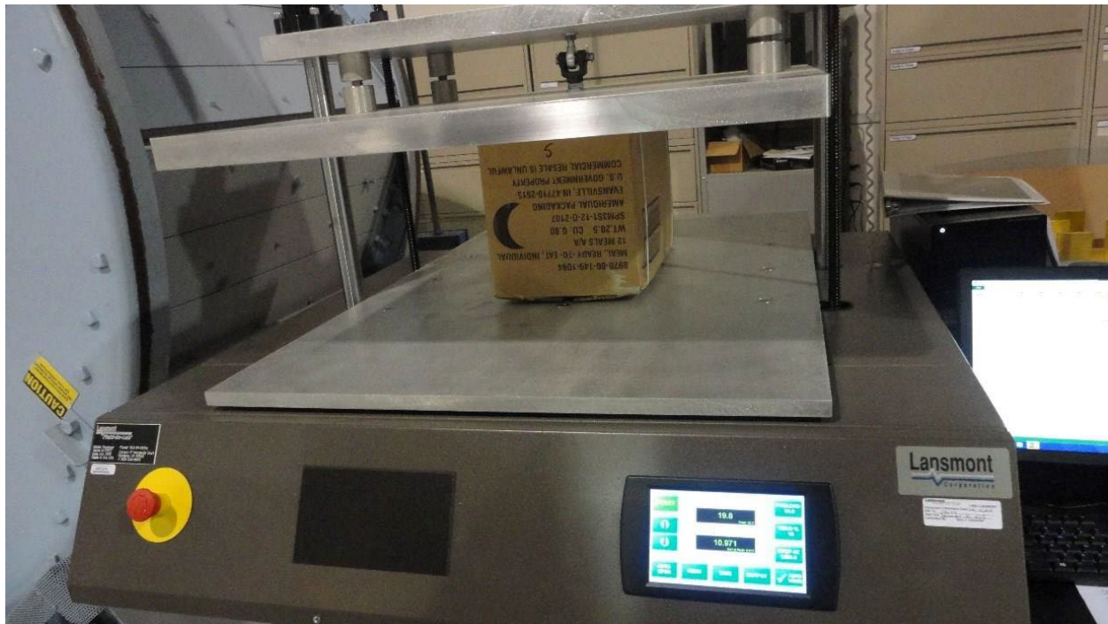
Figure 17. MRE Under Stack Test
