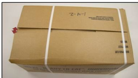
Figure 36. Excessive Gap Width Greater than \frac{3}{4} of an inch. May indicate loose flaps or adhesive failure. Note: Only seen in full inspection of pallet.
