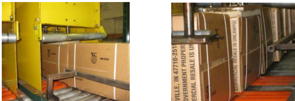
Figure 72. Deflection of cases caused by the pressure of the case staggering system
