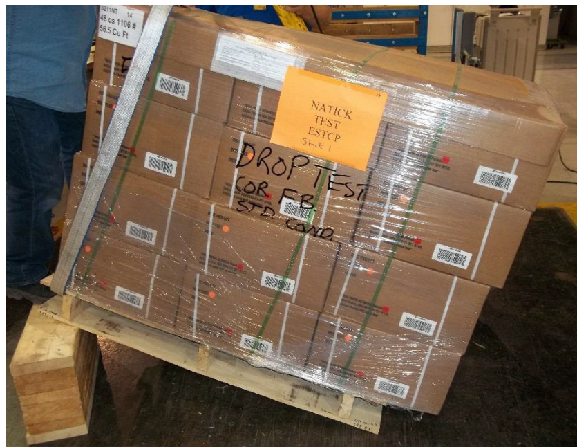
Figure 14. Rotational Corner Drop
