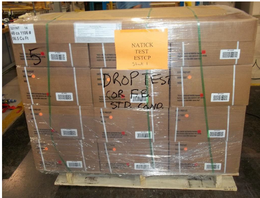
Figure 88. Corrugated Fiberboard Unitized Load (Standard Conditions) Following Rotational Drop Tests
