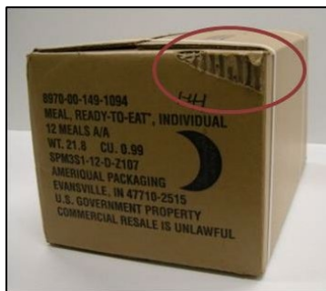
Figure 35. Separation of Fiberboard Layers Delamination or Peeling. Inner layers are visible.
