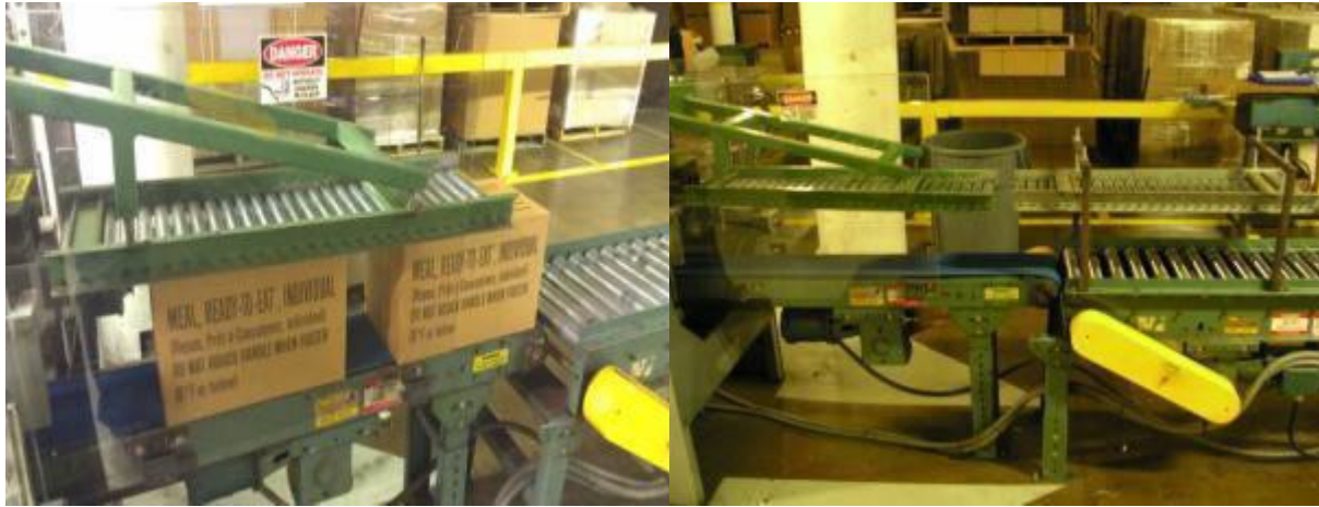
Figure 71. Case sealer prior to (left) and after (right) the closure seal modification
