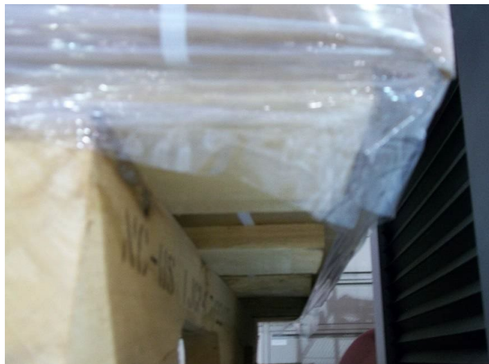
Figure 87. Solid Fiberboard Case Deformation (High Humidity Conditions)
