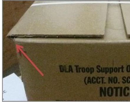
Figure 37. Flaps Pushed Out. Flap does not conform to corner of the case. Most likely will also result in excessive gap width.
