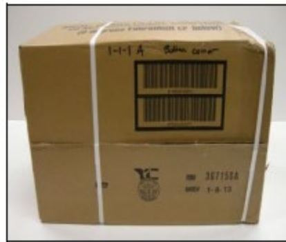
Figure 125. Crushing of the bottom cases that interface with the wooden pallet, overhang will often intensify this type of defect and may also negatively impact compression strength and unit load stability
