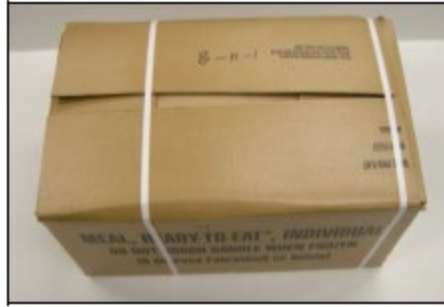
Figure 126. False scores on major flap caused by over-packing of case
