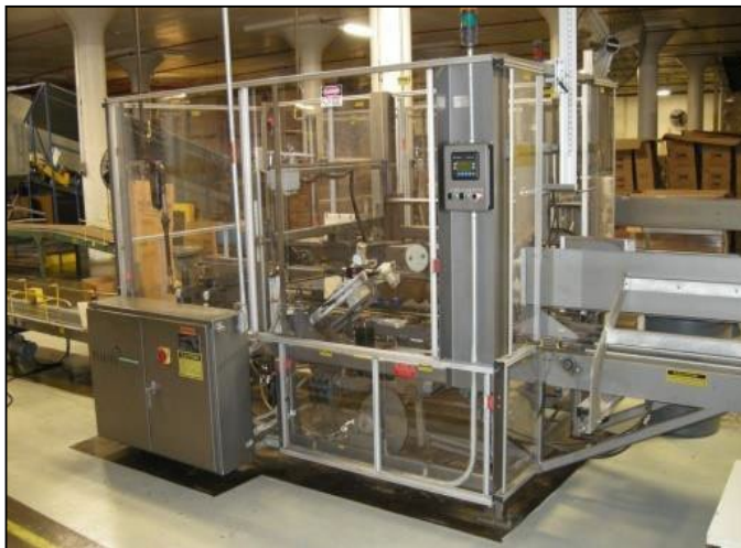
Figure 56. Full view of the case erecting equipment from Pearson Packaging Systems (left) and close up of the gluing of the case's bottom flaps (right)
