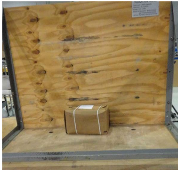
Figure 22. MRE on Loose Load Vibration Table
