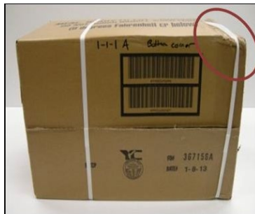
Figure 34. Corner/Edge Crush Crushing, creasing, folding or bending of the fiberboard near a corner or on the vertical edges. It was indicated which one was found in the Observations.
