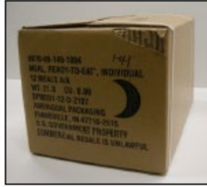
Figure 124. Superficial damage to case during material handling operations or damage from case assembly equipment
