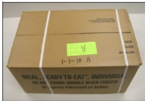
Figure 123. Minor flaps pushed out due to over-packing of corrugated case
