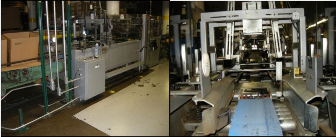
Figure 60. Klippenstein SK500 HM case sealing equipment for the top flaps (left) and view of the front entrance of the equipment (right)
