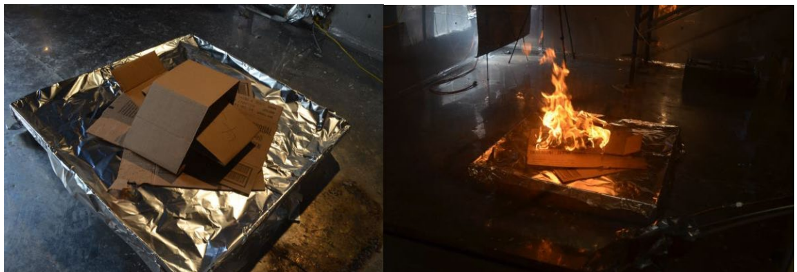
Figure 45. The paperboard test material (corrugated Spectra-Kote Polymer Fiberboard case and liner) atop aluminum foil (left) on 1 \text{ m} \times 1 \text{ m} ( 3.2 \text{ ft} \times 3.2 \text{ ft} .) steel pan. Combustion of same (right)
