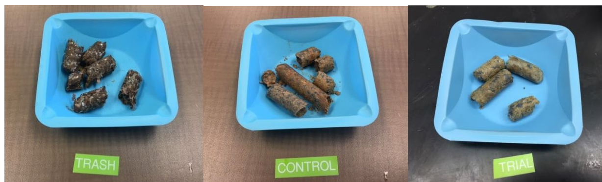
Figure 104. Pellets after filtering out the fines, from left to right: made from 12/5/16 trash, Recipe #2 control feedstock, Recipe #2 trial feedstock
