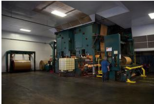
Figure 52. Coating paper with the Spectra-Kote
