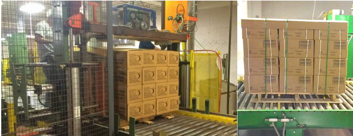
Figure 68. Images of the unitization of current MRE rations (48 cases per load) (left) and a fully-strapped unitized load (right)
