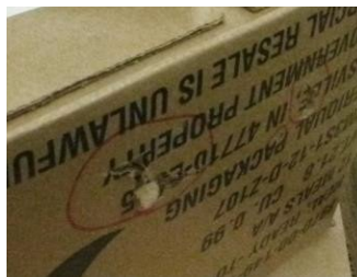
Figure 38. Puncture Hole in case. Any time internal packaging was visible. Any small or large hole in packaging, localized in a circular shape.
