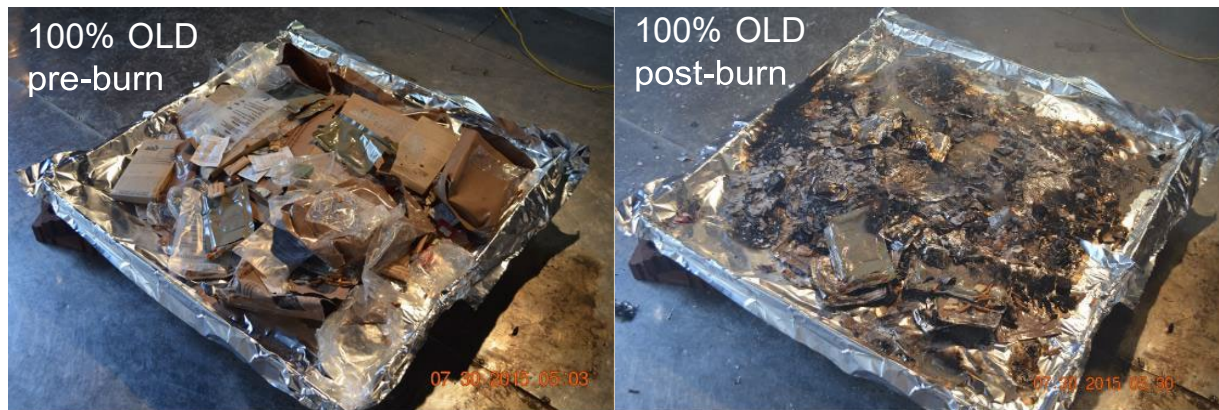
Figure 46. MRE (10 % OLD material or 0% NEW) on 3.2 × 3.2 foot steel pan, before (left) and after (right) burn
