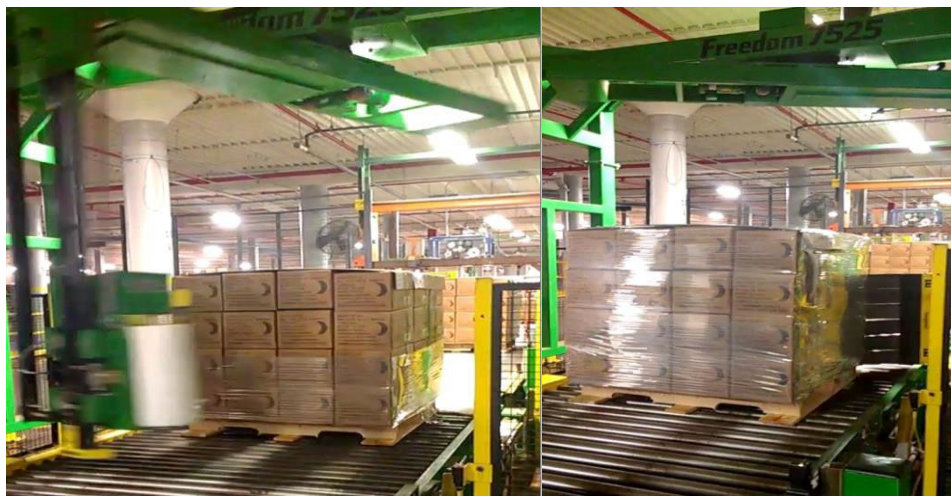
Figure 69. Stretch wrapping operations of unitized loads (automatic rotary arm stretch wrapper)
