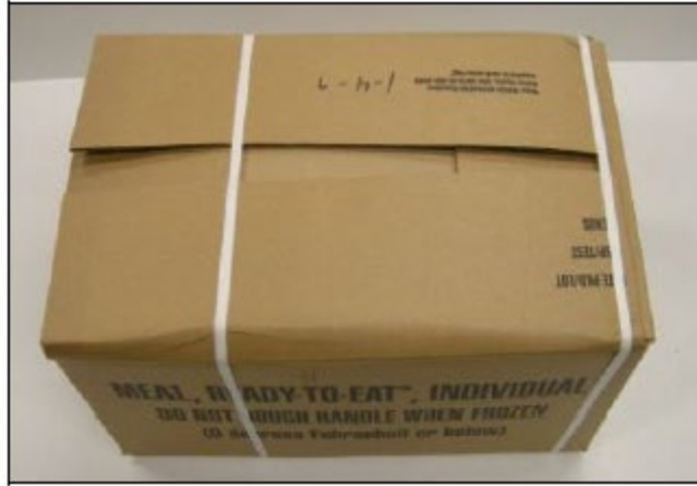
Figure 122. Misaligned straps due to the larger case size, issue can be corrected through adjustment of strapping systems
