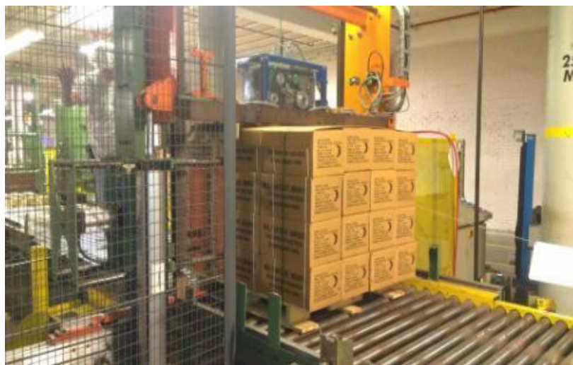
Figure 74. Pallet strapping unit (three straps per pallet)
