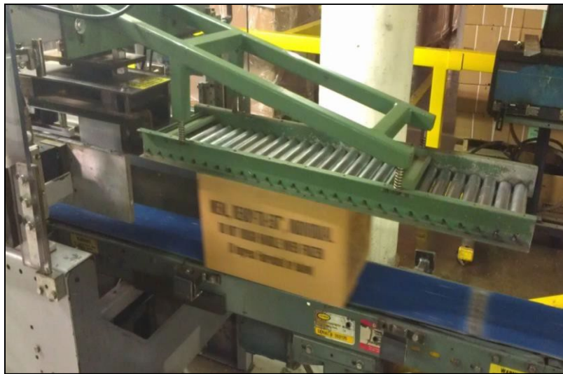
Figure 61. Conveyor system used for securing glued flaps during curing of adhesive
