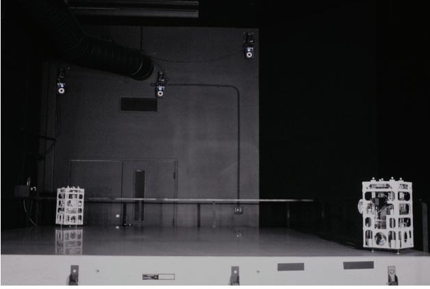
Figure 2: NPS-POSEIDYN testbed with the Vicon motion capture cameras, FSSs, and granite monolith in the Spacecraft Robotics Laboratory at the Naval Postgraduate School. The Target FSS is on the right and the Chaser FSS is on the left.
