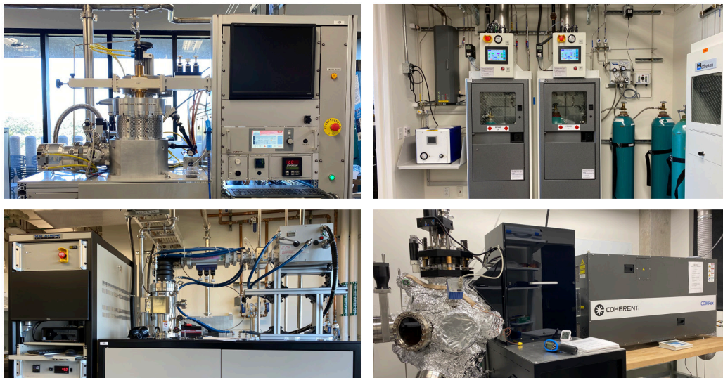
Fig. 2 Diamond growth microwave-plasma CVD (MPCVD) systems, PLASSYS SSSDR-150 (top left) and SEKI SDS6350 (bottom left), have been installed at the facility. (top right) The gas safety cabinets for H 2 , methane (CH 4 ), and ammonia storage. (bottom right) The Pioneer 180 PLD equipment and the COMPEX 205 excimer laser.
