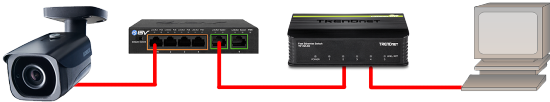
Figure 14: Camera connected to desktop computer. Red lines indicate Ethernet cable connections [30][93][94][95]
