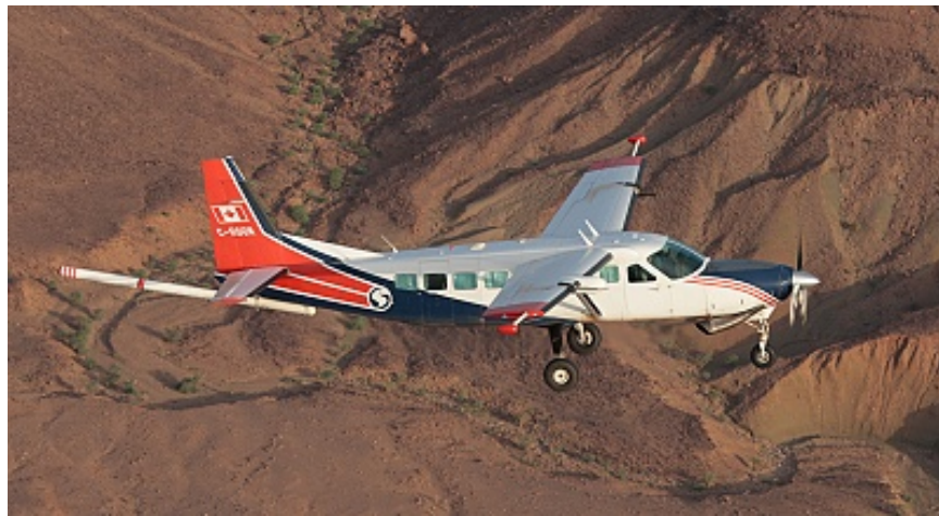
Figure 6: Tail mounted stinger on survey aircraft. [11]
