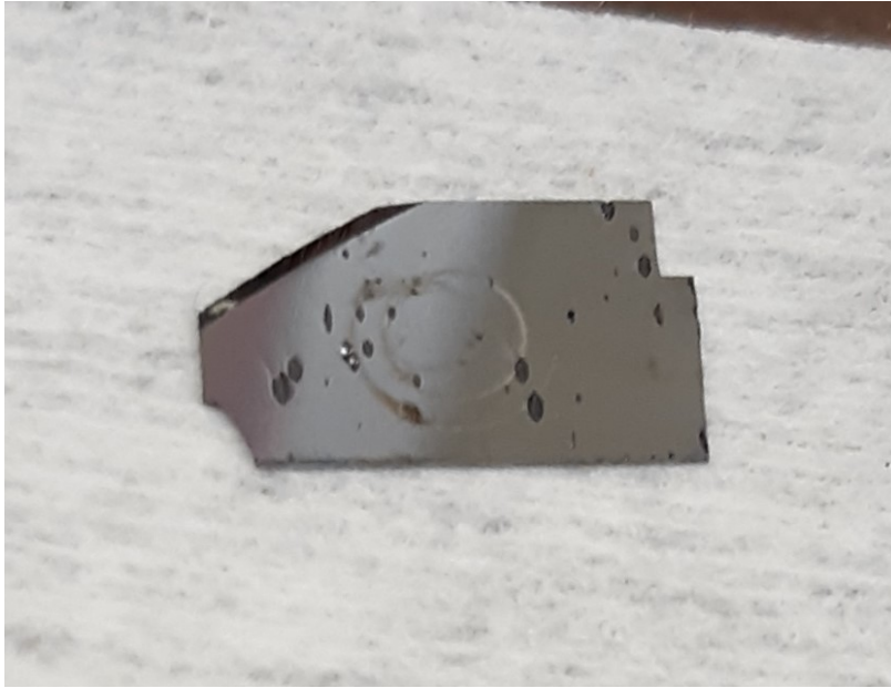
Figure 61: Picture of damaged GaAs 0.602 P 0.398 sample. Note the two circular damage patterns, which occurred while irradiated with 300 mW (outer) and 150 mW (inner) of average power. These rings appear on both sides of the sample, even though the pump was only incident on one side of the sample.
