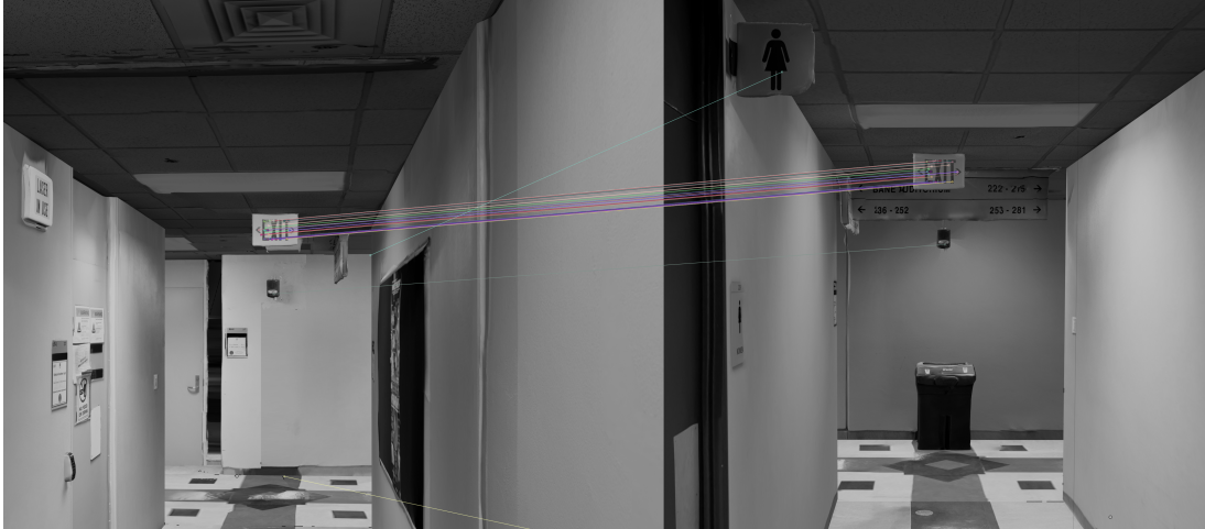
Figure 3: Feature matches occurring between different exit signs
