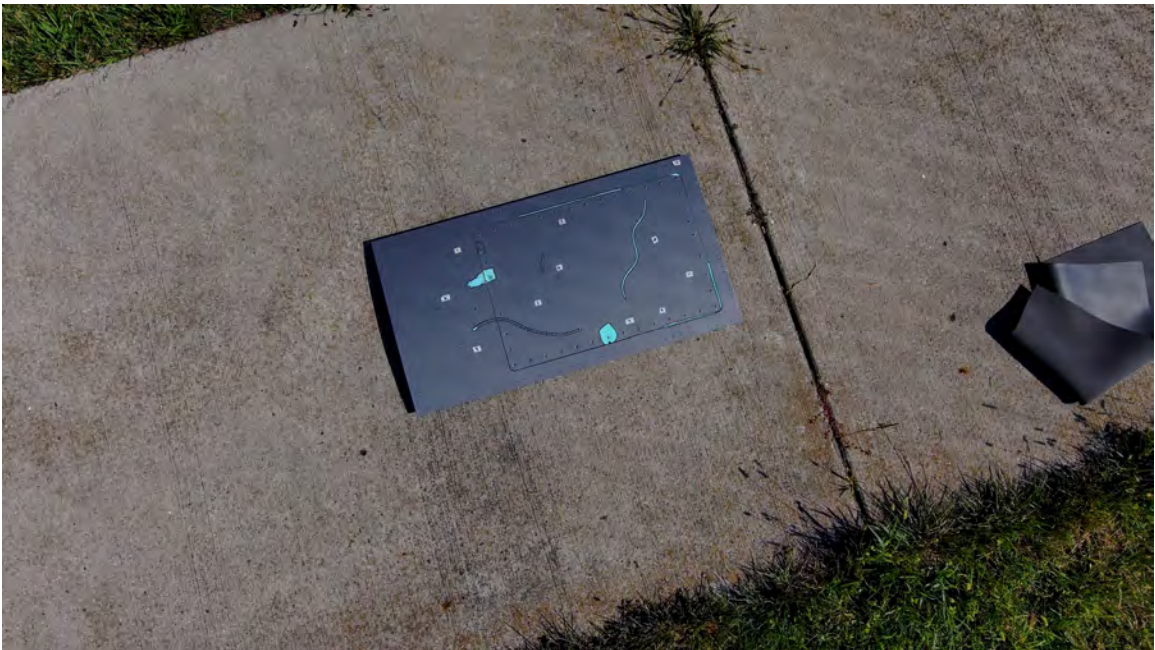
Figure 14: Aircraft Panel with Surface Flaws for Pixel Size Determination, 2m
