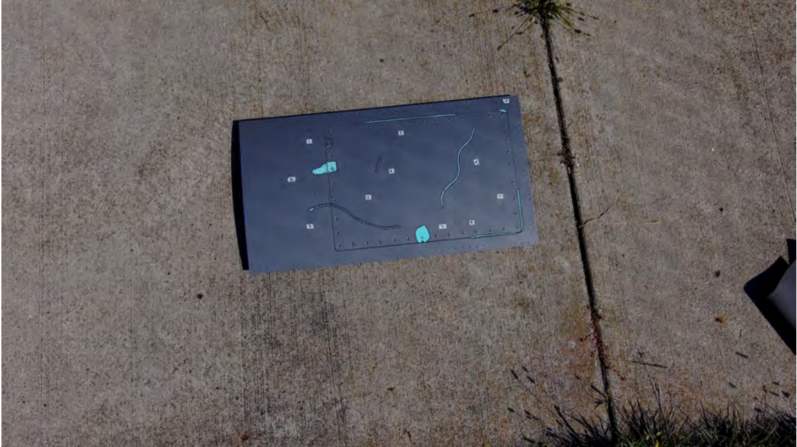
Figure 13: Aircraft Panel with Surface Flaws for Pixel Size Determination, 1m
