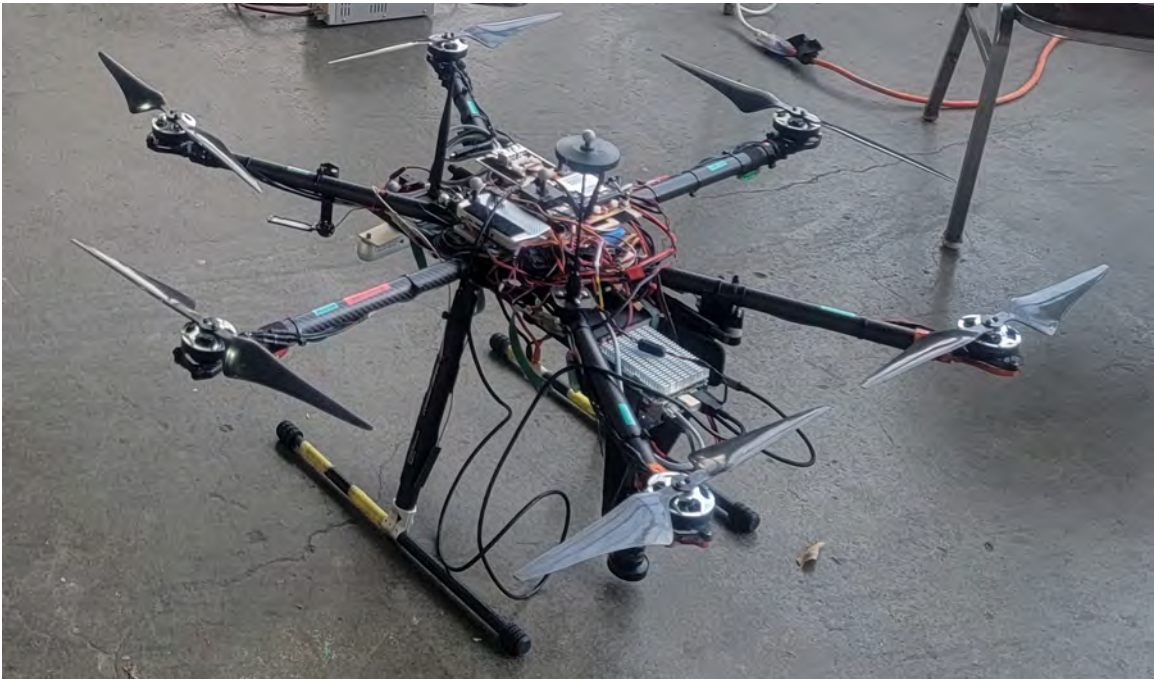
Figure 4: Hexrotor with camera mount in Hangar
