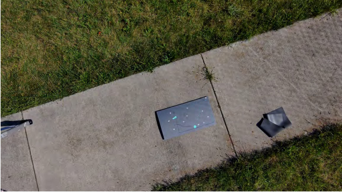
Figure 15: Aircraft Panel with Surface Flaws for Pixel Size Determination, 3m
