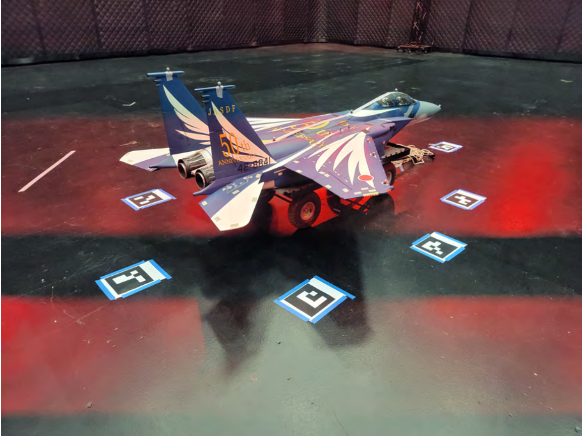
Figure 16: 1/7 Scale F-15 Model with ArUco tags in Vicon Chamber
