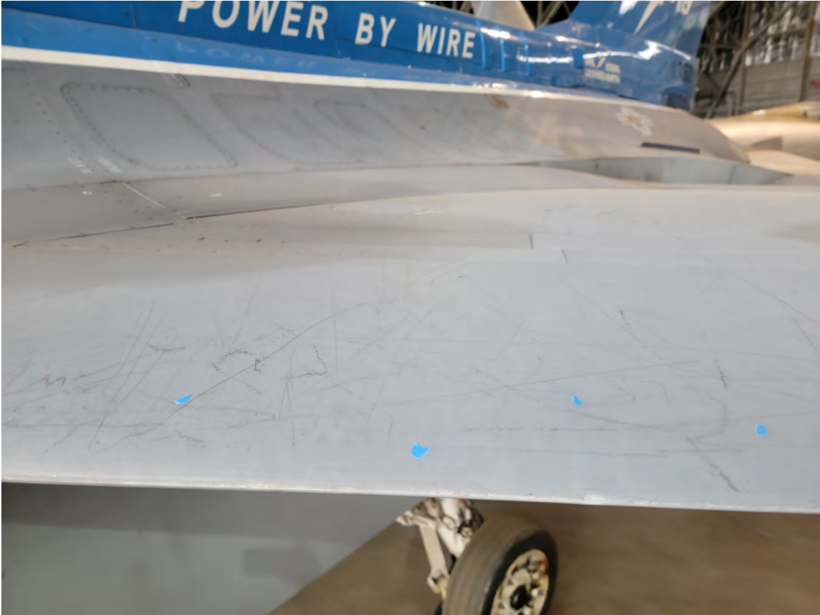
Figure 40: F-16 Surface Flaws On Leading Edge Ground View
