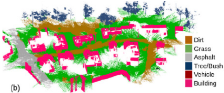
Fig. 1 Dense metric-semantic 3-D mesh model of an urban scene generated by Kimera-Multi with three robots
