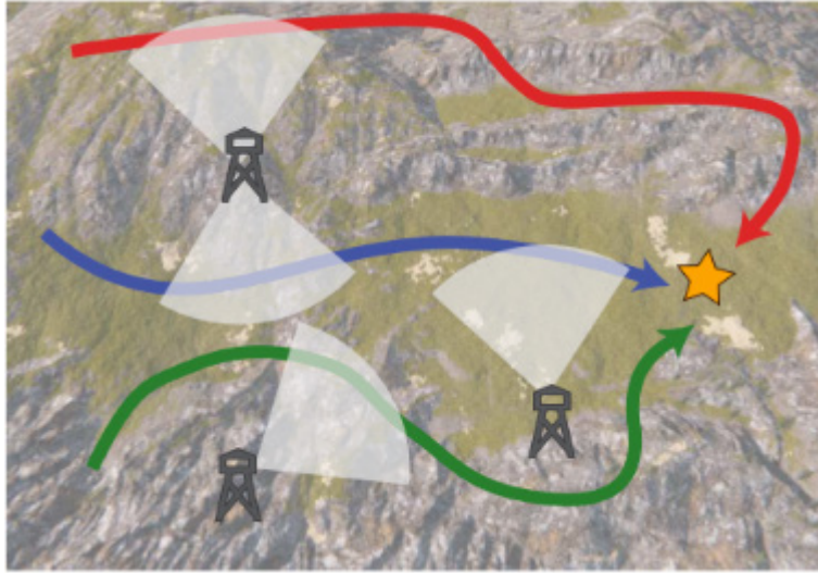
Fig. 32 Example of different paths with different detection likelihoods taking into consideration terrain geometry
