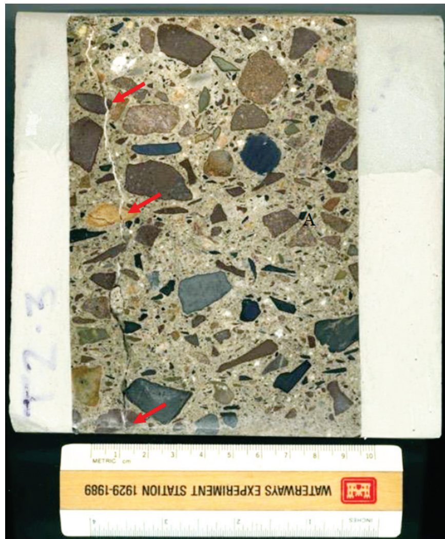
Figure 41. Polished cross section of core T2-3 with locations of cracking through aggregates indicated.
