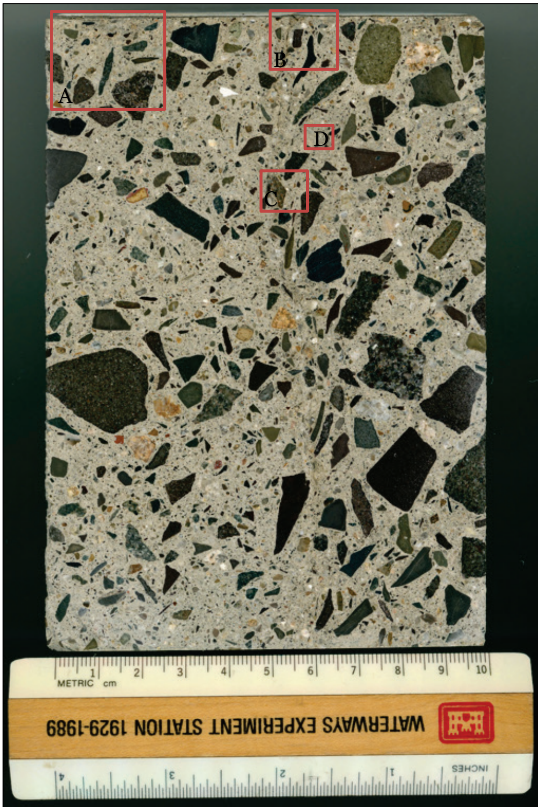
Figure C3. Scanned image of polished sections from core T1-S1. Lettered boxes refer to locations of micrographs in Figure 4.
