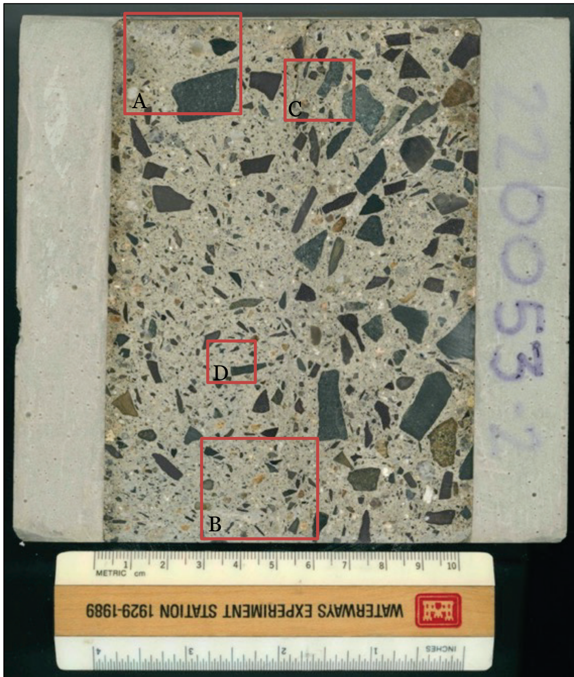
Figure C10. Scanned image of polished sections from core T1-S2. Lettered boxes refer to locations of micrographs in Figure C11.
