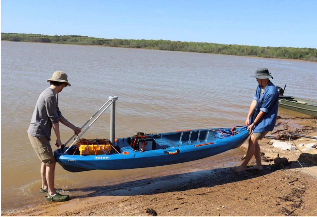
Figure 20 - Kayak with data collection system installed
