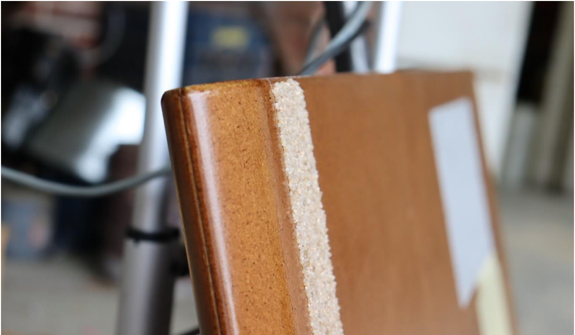
Figure 19 - Turbulence trip strip.
