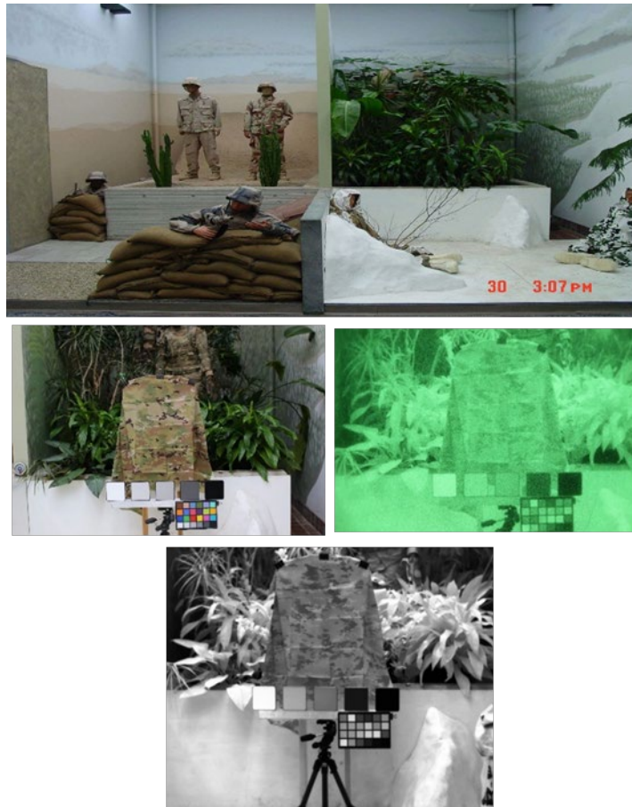
Fig. 1 To touch the complexity of signature control for a dismounted Soldier, one must address the relationship and interactions of the EM spectrum (VIS, NIR, and SWIR) mapped onto the Soldier in a multidomain operational environment (image provided by DEVCOM SC)
