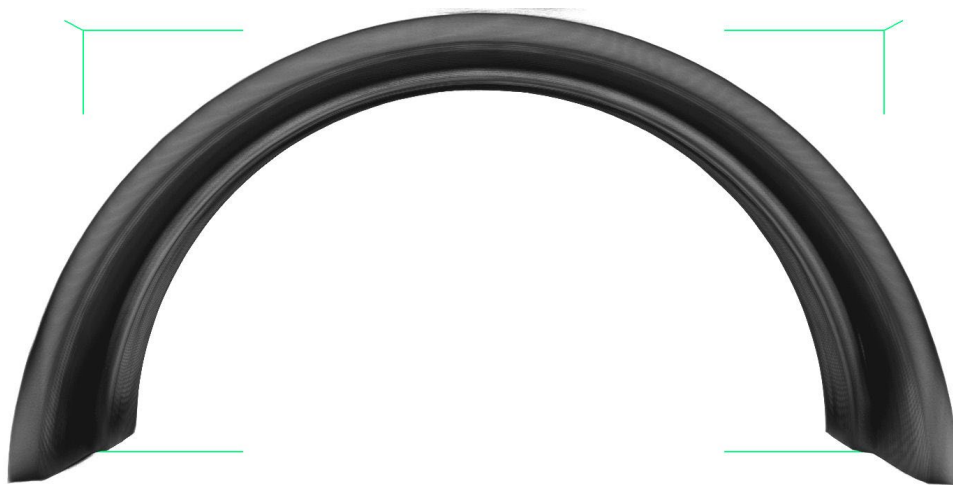
Fig. 8 Outside 3-D solid image of the half-ring specimen, in which some of the dark air artifact is apparent in the middle area of the half ring from one end to the other
