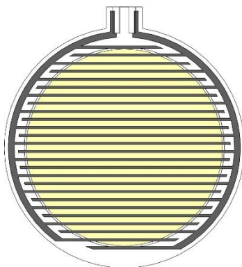
Figure 2. Designed BN ion gate at a 3 mm cross section height.
